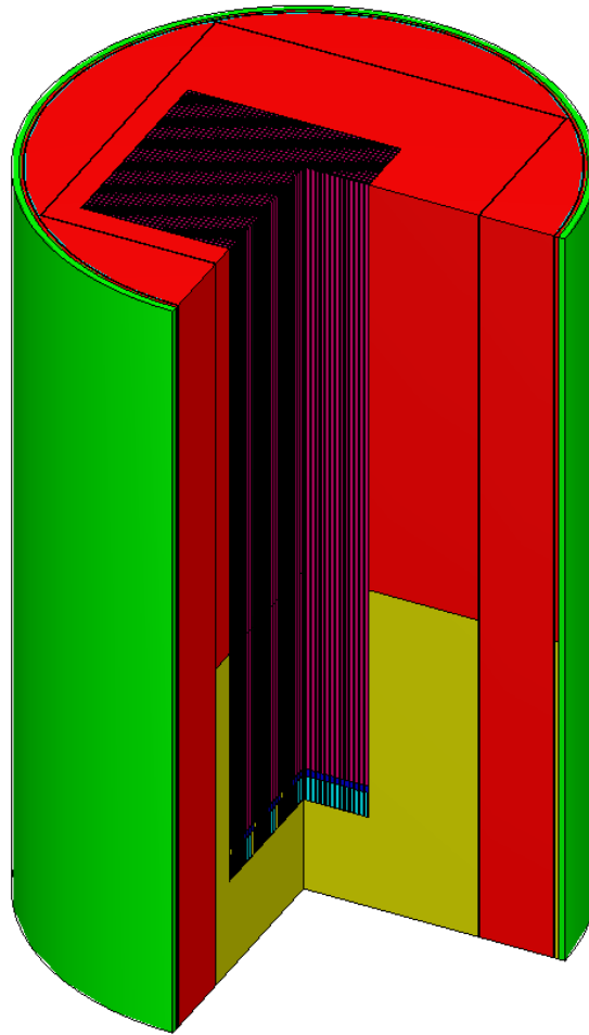
Figure 8.8: Cut-away of KRITZ-2:1 core done in KENO 3D.
