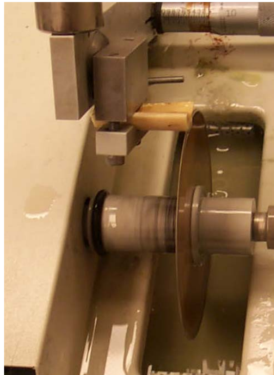
Figure 4-14. Buehler® Isomet™ low speed saw used to make thin sections of cortical bone samples.
