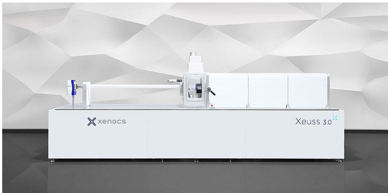
Figure 2.12 X-ray scattering equipment. The left part is the X-ray beam generator. The right part is the sample and detector.
