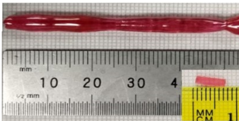
Figure 3.2: An as-grown crystal boule of \text{Er}_2\text{Be}_2\text{SiO}_7 and a small oriented crystal grain.
