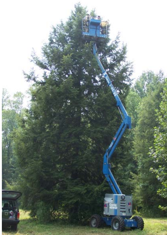
Figure 5. Collection of eastern hemlock branches using an articulating boom (Genie Z 45/22, Tigard, OR).
