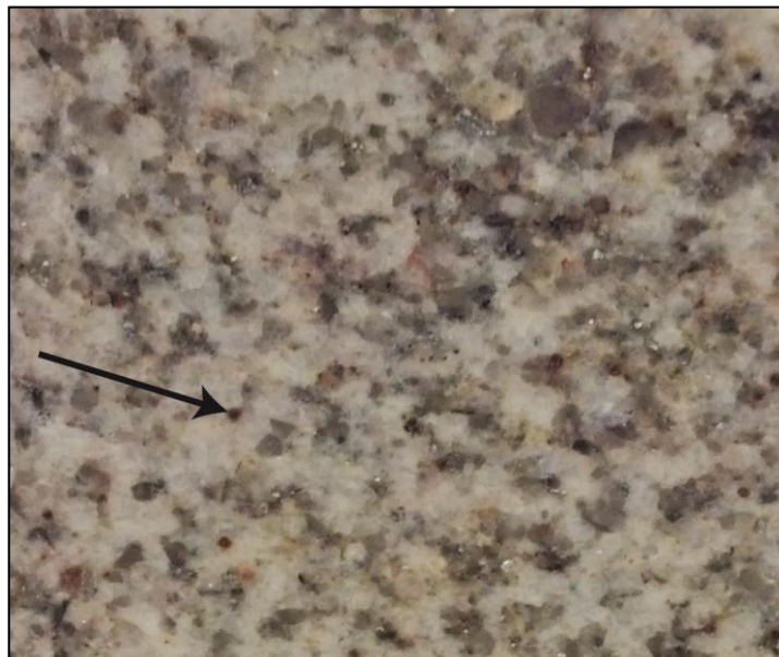
Figure 5-2. Sample HBC10-55 (see Fig. 3-3 for location) showing fine grained homogeneous CMG representative of the Curecanti pluton core; arrow is 1 centimeter-long and identifies a subhedral magmatic garnet.
