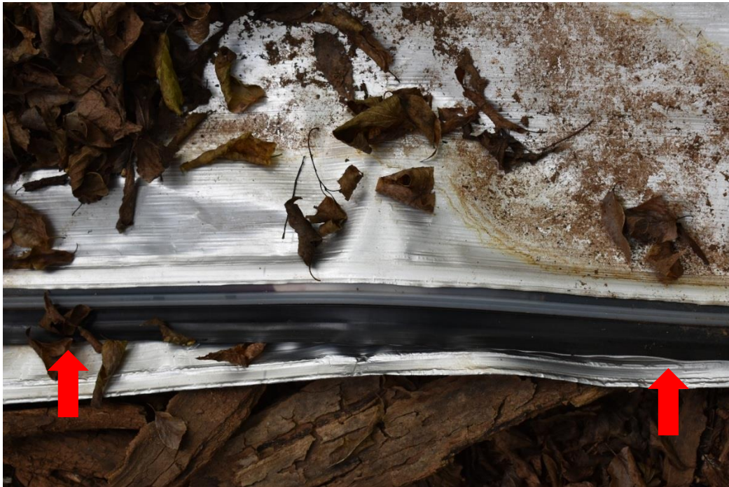
Figure 6.9 Experiment 1.1: Blood Pressing on Seal of BBB (where red arrows point)
