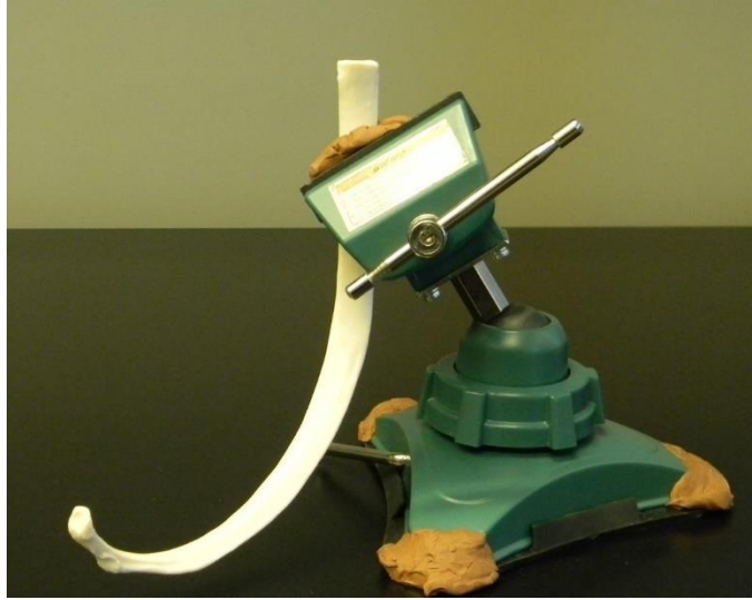
Figure 4: Rib orientation and clamping system
