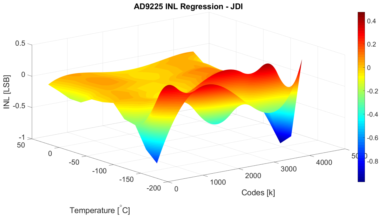
Figure 3.30: AD9225 INL Regression Using JDI Ramp Data
