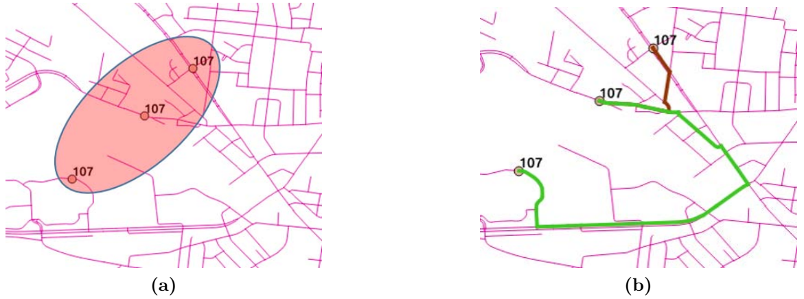
Figure 3.1: Incorrect clustering by K-means, because of the ignorance of underlying road network.
