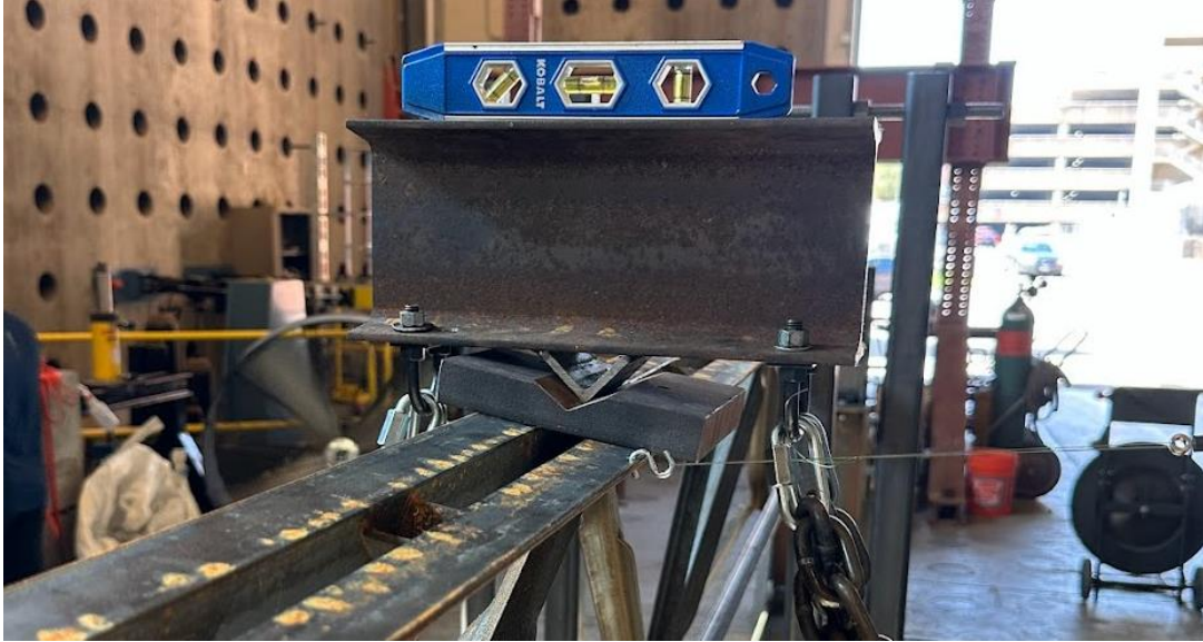
Figure 11. Knife Edge for In-Plane Bending Experiments
