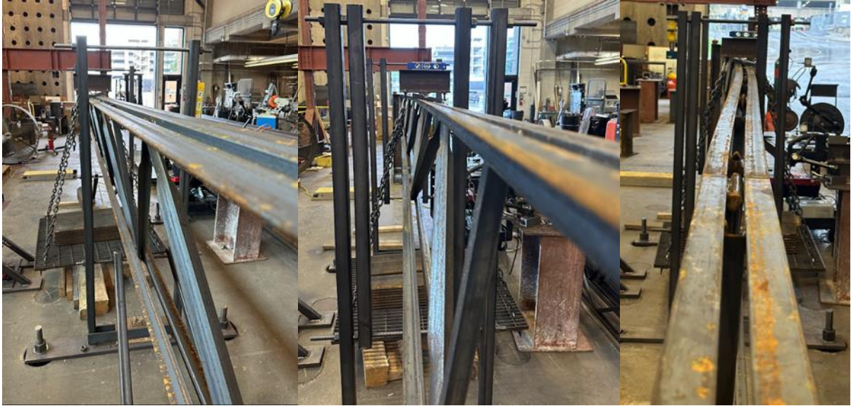
Figure 15. Photos of Deflected Joists
