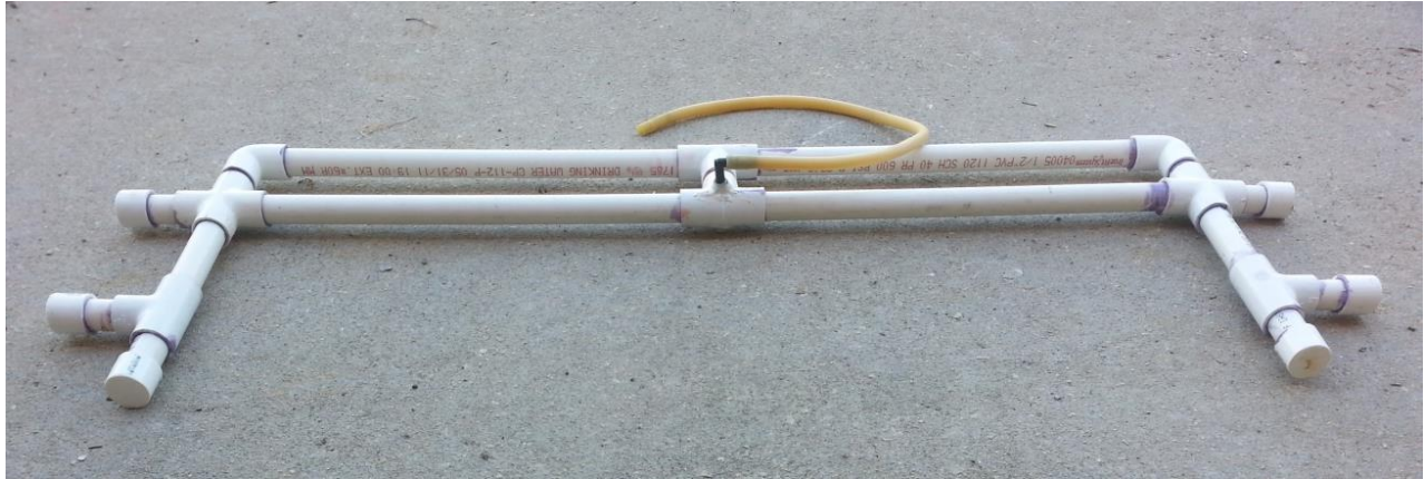
Figure 21. Second generation sequencing batch reactor decanter.
