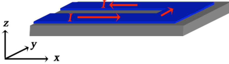
Figure 2.10: Geometry of the piezoresistor on the cantilever adapted from Ref. [29] with direction of the current shown.
