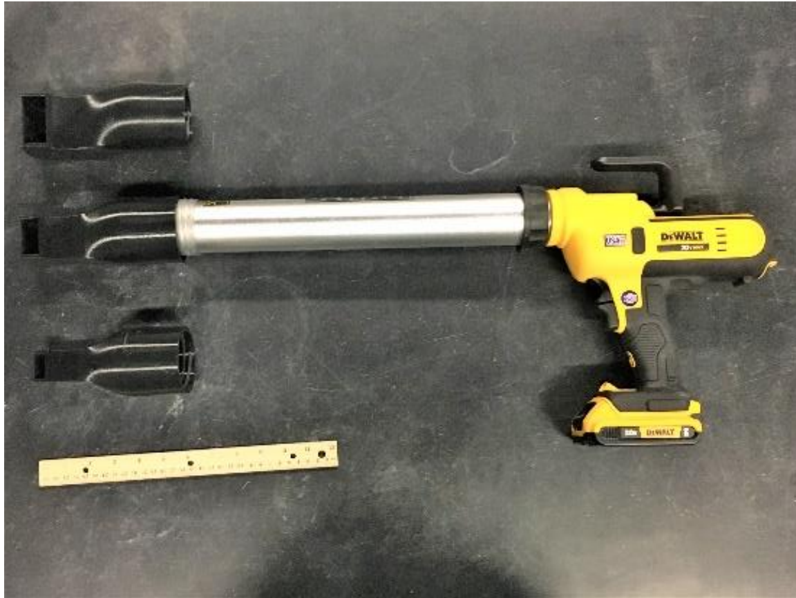
Figure 25: Caulk gun and nozzles ( 2 \times 1 in., 1.5 \times 0.75 in., and 1 \times 0.5 in.) used to fabricate the multilayered printed concrete specimens.
