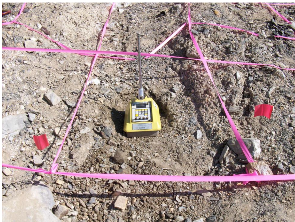
Figure IV.2 Nuclear Density Gauge Testing on Reclaimed Mine Slope
