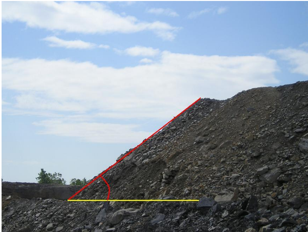
Figure IV.20 Example of Measured Angle of Repose at National Coal Site
