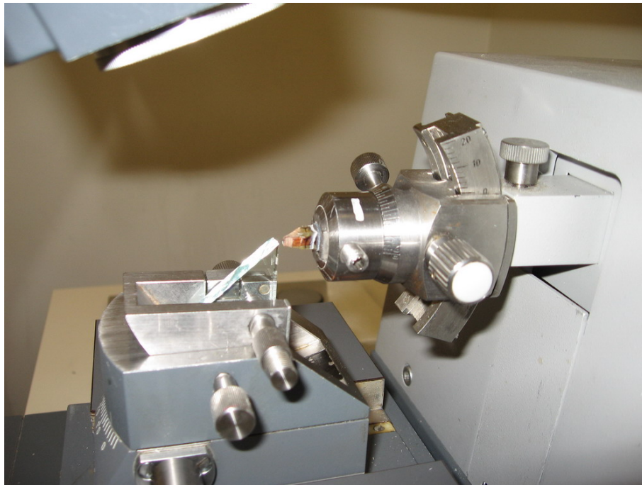
Figure 3-3. Process of microtoming
