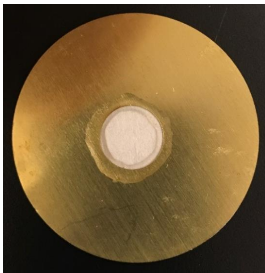
Figure 2.2 A photo of a testing membrane sample. The membrane is typically mounted on a brass disc and the edge is sealed using epoxy.
