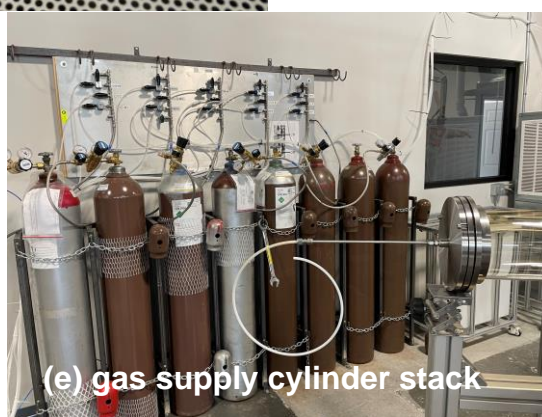
Fig. 2.6 Thermal CVD experimental setup at General Graphene (a) CVD experimental setup, (b) CVD quartz tube, (c) sample holder, (d) CVD gas flow control valve and computer control unit, (e) gas supply cylinder stack
