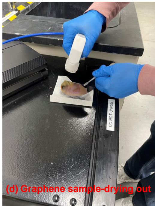
Fig. 2.8 Surface cleaning/rinsing of the CVD-graphene sample (a) Graphene on Si substrate after overnight drying, (b) Graphene sample in acetone bath (5-10 minutes), (c) Graphene sample in Iso-propyl alcohol (IPA) bath (5-10 minutes), (d) Graphene sample (drying out)
