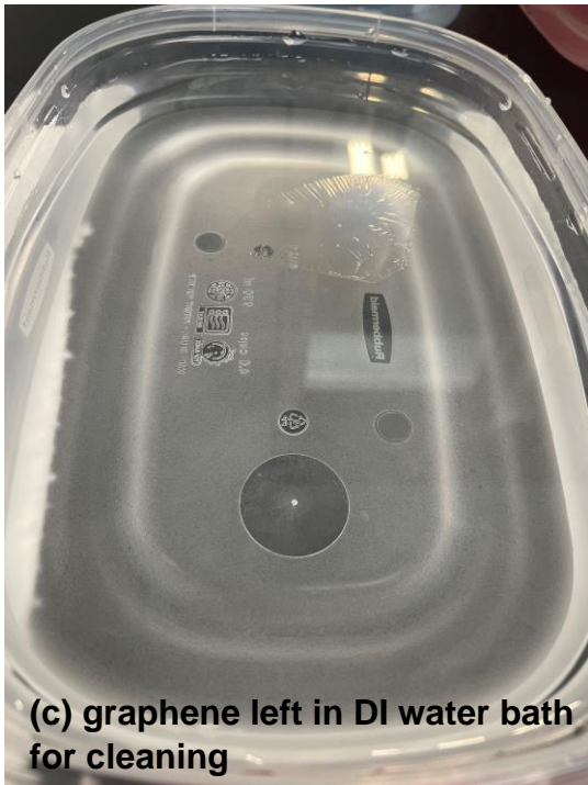
Fig. 2.7 CVD graphene sample etching (a) in ammonium per sulphate (APS) solution and wet transfer process (b-d) onto new SiO 2 /Si wafer
