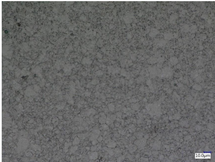
Fig. 2 Optical image of graphene grains growth in regions of high Cu at.% of \text{Cu}_x\text{Ni}_{1-x} alloy film on \text{Si}/\text{SiO}_2 substrate showing discoloration and small sized grains-silicide formation
