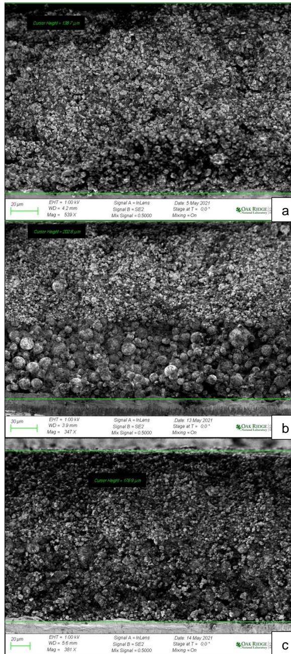
Figure 13. SEM microstructure of each cathode configuration, a) all small configuration, b) large particle size followed by small particle size configuration, and c) mixed particle size followed by small particle size configuration.
