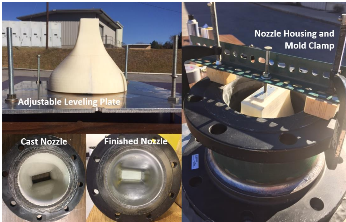
Figure 27. Nozzle contraction casting.
