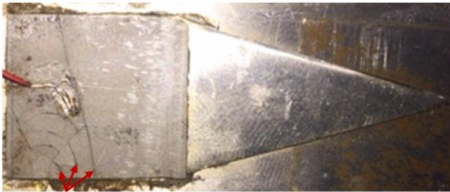
Figure 15. Example of stress cracks in an actuator.
