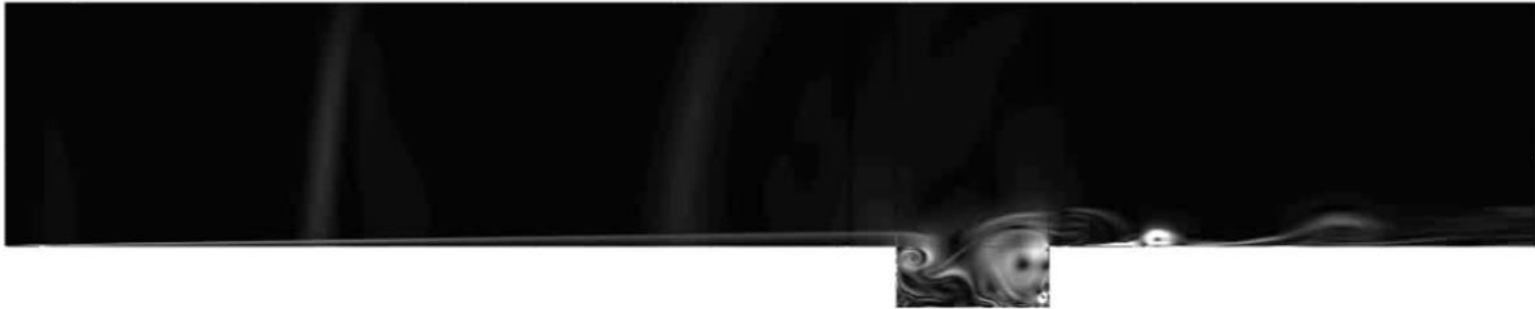
Figure 55. Cavity flow field visualization using the magnitude of the density gradient illustrating the cavity flow field, the forward-propagating wave, and the turbulence downstream of the cavity.
