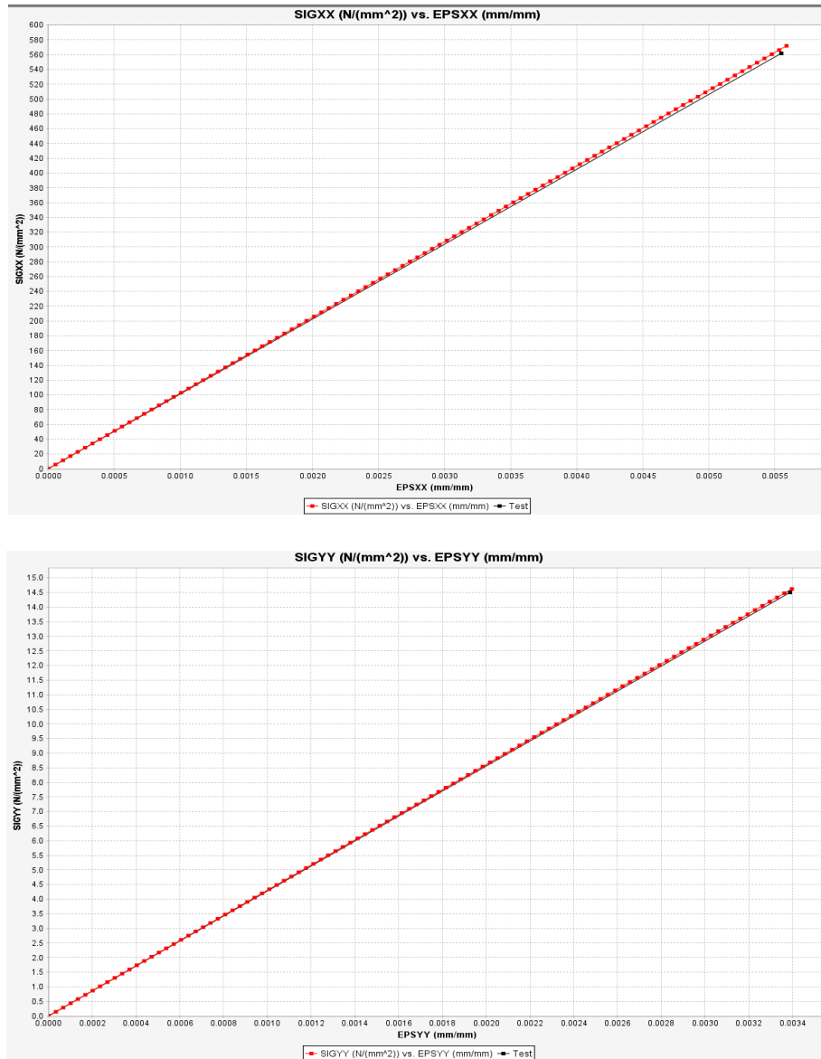
Figure 4.4: A correlation between the tensile strength of epoxy sized TCF-TSU composites in longitudinal (SIG XX) and transverse (SIG YY) direction: simulation (red color) vs. experimental (black color) results at 0.53 \mu\text{m} interface thickness
