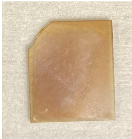
Figure 37. A polished LISe sample before being chemically etched. The interferometer results for the Y-profile (vertical) of this sample can be seen in Figure 36.
