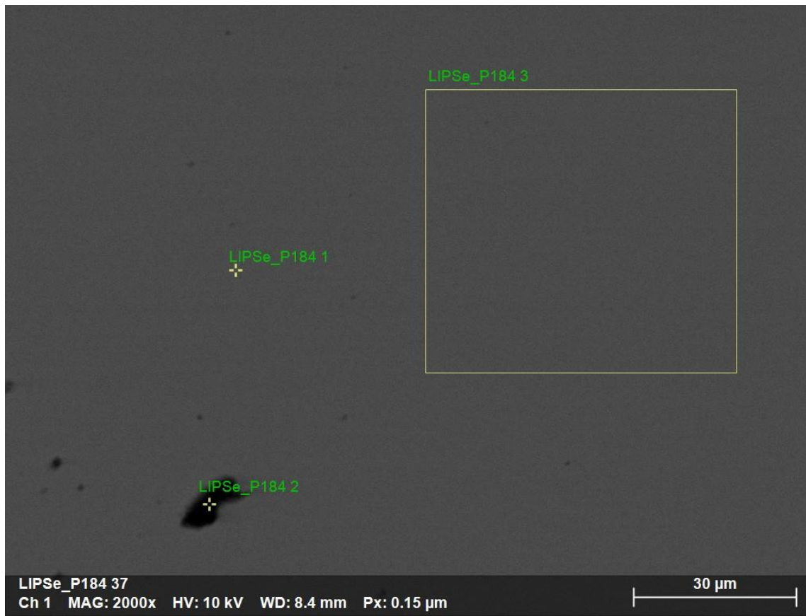
Figure 51. SEM image of a LIPSe sample with 10 nm of SiO 2 sputtered on the surface. SEM-EDS measurements were taken at the three regions identified above. SEM-EDS does not measure lithium content.
