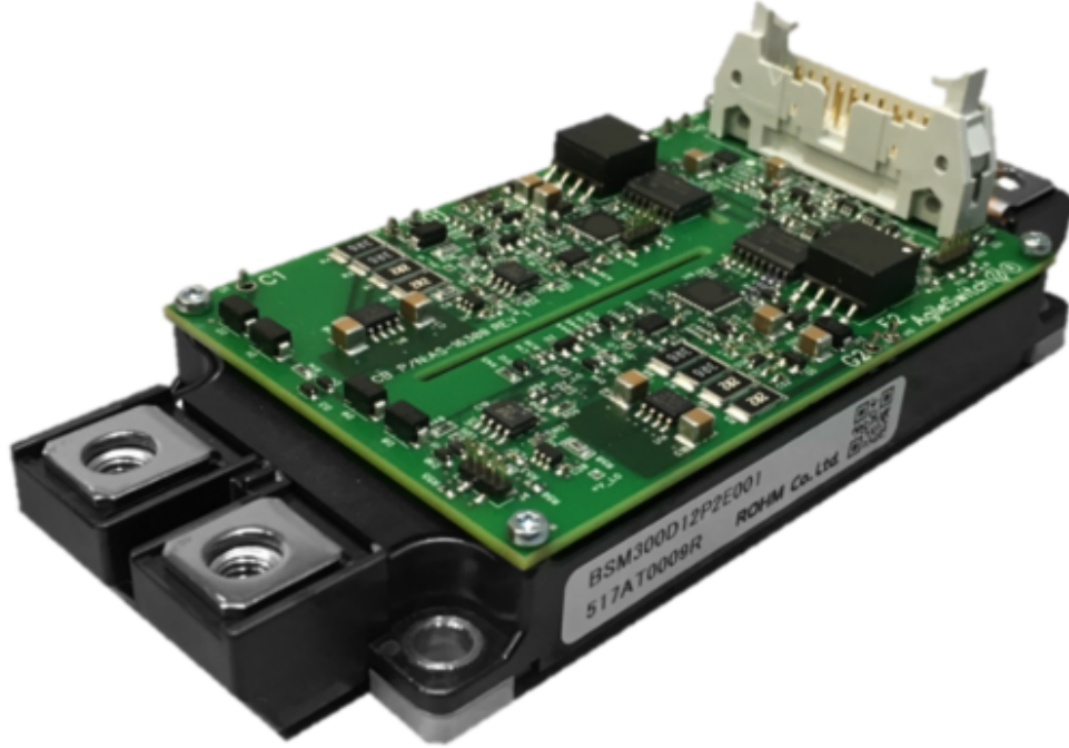
Figure 1.4: AgileSwitch intelligent gate driver on top of SiC power module [13]
