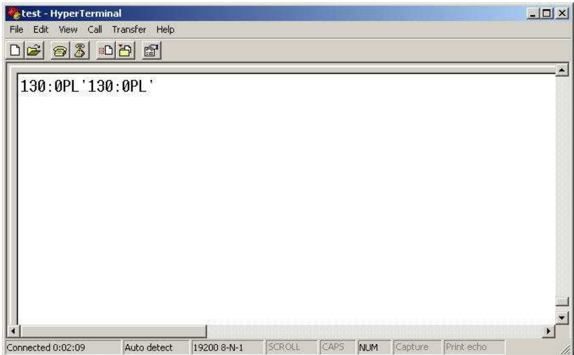
Figure 4.13: Hyper-terminal receiving the MODBUS read packet after 2 minutes
