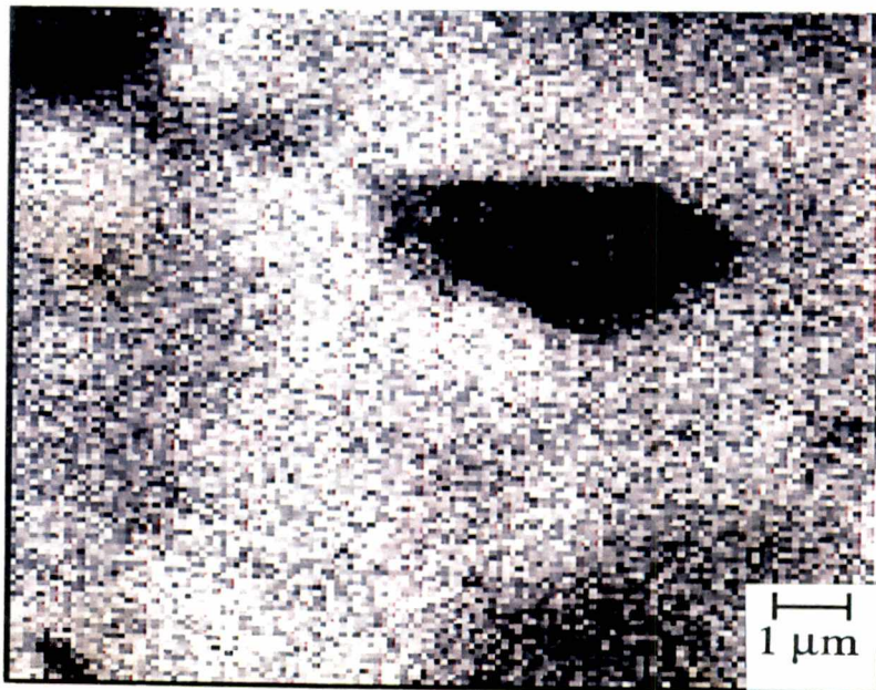
Figure 4.26. Auger mappings of metallic aluminum (a) and nitrogen from AlN (b) in AlN substrate laser-irradiated with 1 \text{ J/cm}^2 in Ar-4% \text{H}_2 .
