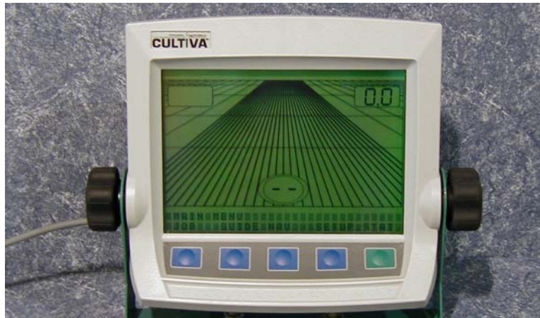
Figure 3.3. Cultiva Marker™ equipped with a graphical display to provide guidance information to the operator.
