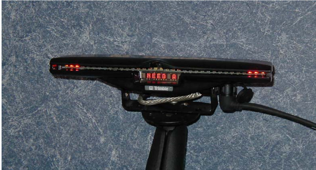
Figure 3.1. Trimble AgGPS@21 lightbar equipped with a single row of LED's to provide guidance and correction information to the operator.
