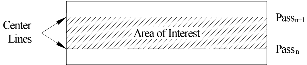
Figure 3.13. Illustration of area of interest when calculating percent overlap or skip between pass n and n+1 .
