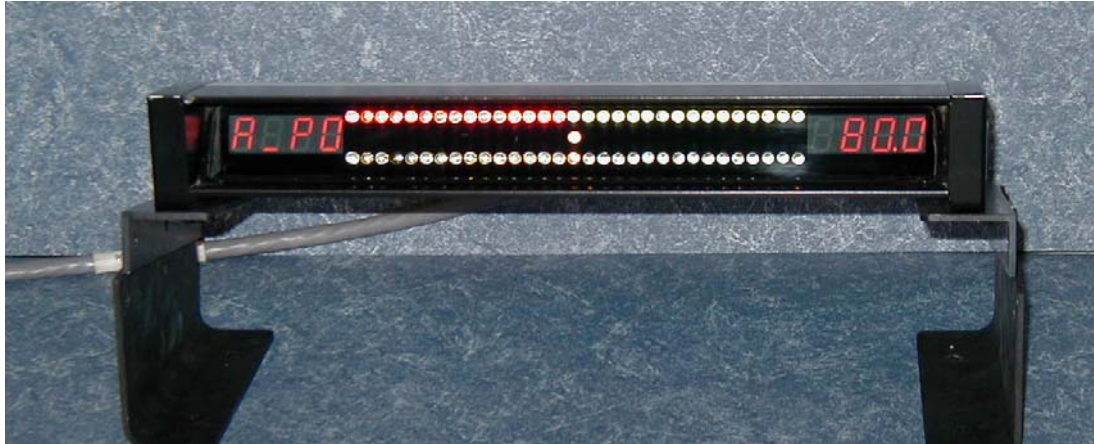
Figure 3.2. Satloc LiteStar equipped with double row LED's and 7-segement displays to provide guidance and operation information to the operator.
