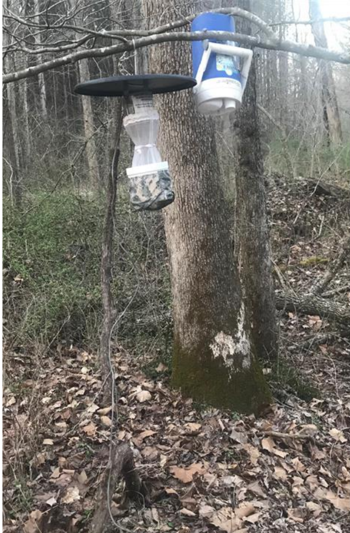
Figure 2.3. CDC light traps (CO 2 ) used for insect sampling at Arnold Air Force Base, 2022 and 2023.
