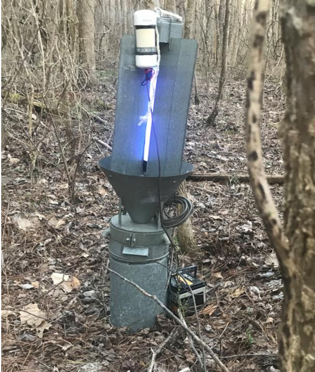
Figure 2.2. Ultraviolet (UV) light trap used for insect sampling at Arnold Air Force Base, 2022 and 2023.
