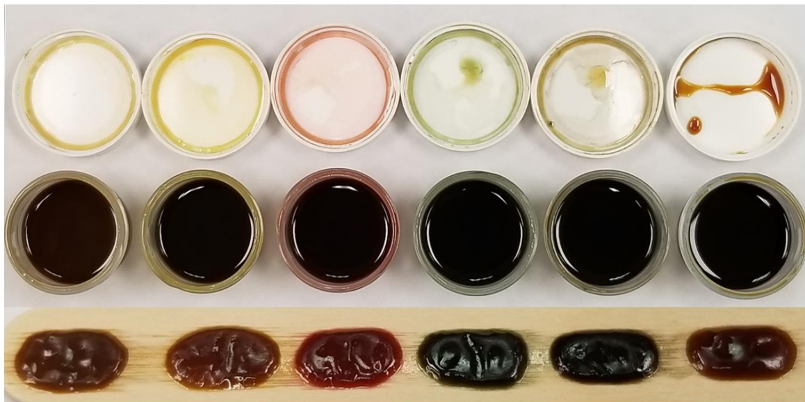
Figure 16. Lignin resins pigmented (left to right) white, yellow, red, blue, black, none.
