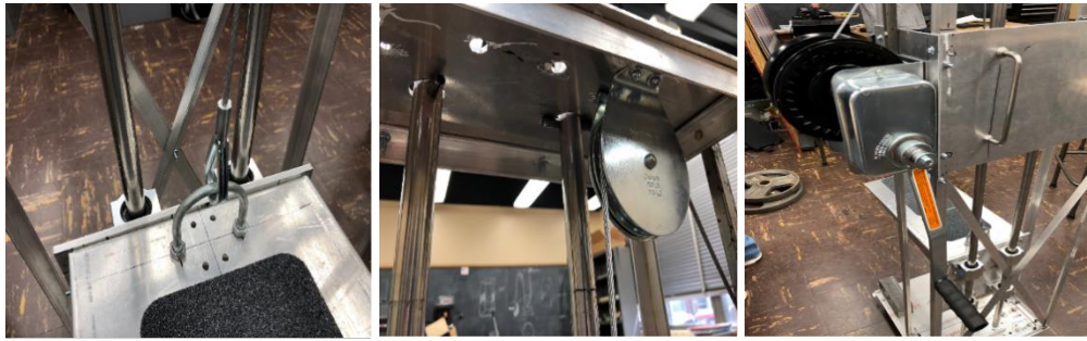
Figure 1a,1b,1c. U-bolt Attachment to Fork, Pulley with Cable, Winch Bolted to Frame
