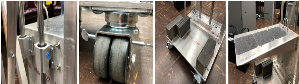
Figure 2a,2b,2c,2d. Linear Sleeve Bearings, Pivoting Front Castors, Base plate and Counterweights, Lifting Fork
