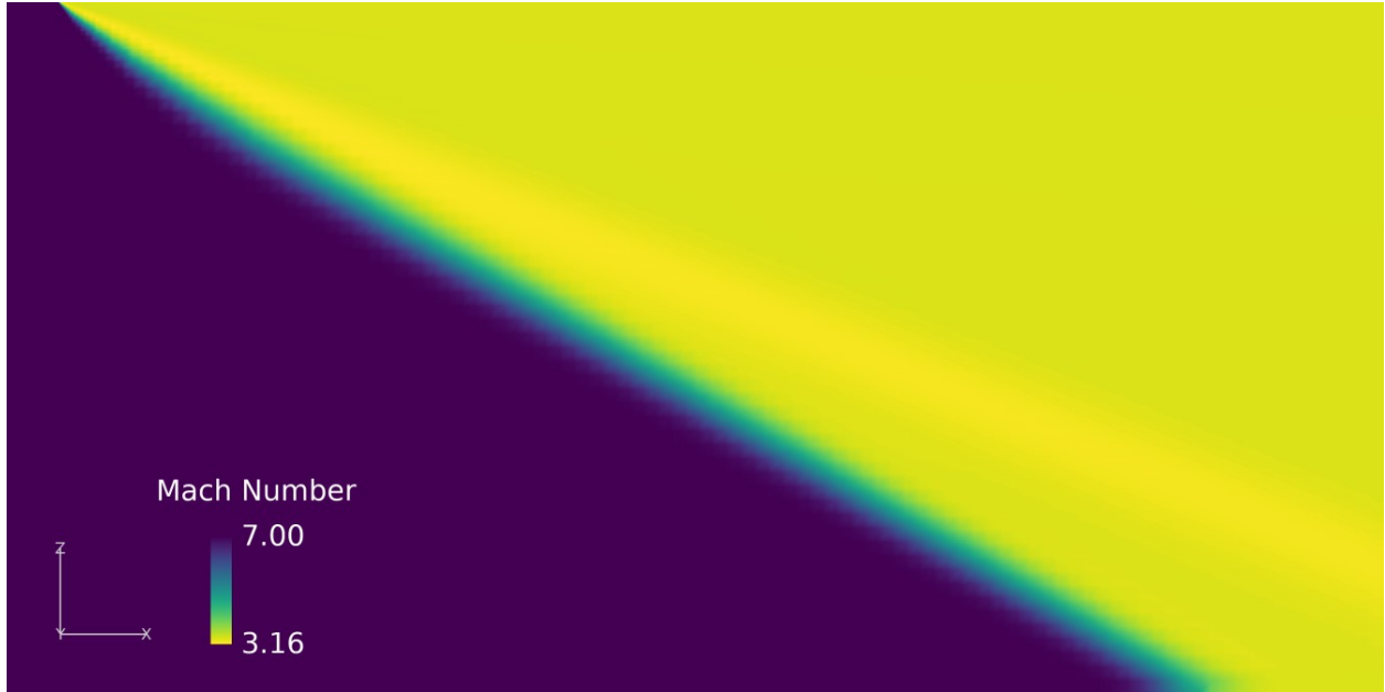
Figure 16: Mach Number for 30° Oblique Shock Created by Top Boundary Condition
