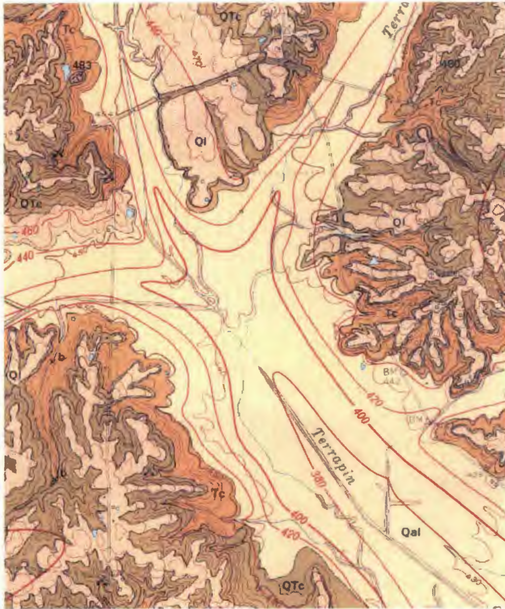
Figure 3: The nature of under fit streams and associated valleys and interfluvies found in Western Kentucky. C.I.=3.05m. Contours drawn in red are proposed contours found on erosional surfaces of Eocene aged rocks. Source: Lambert, 1965. (Approximate scale 1:23,200. C.I.= 3.05m).
