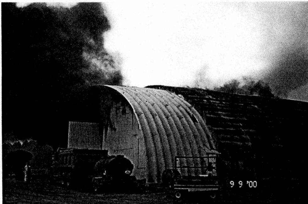
Figure B-23 Outside View of Aircraft Shelter Used for Composite Wing Burn Test with Small JP-8 Fuel Fire Inside.
