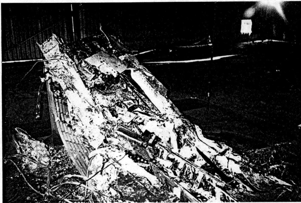
Figure B-22 Post Burn Fire Damaged Composite Wing Structure.
