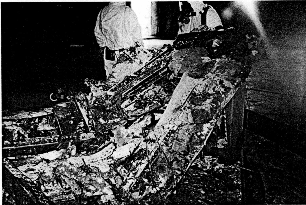
Figure B-24 Close-Up of Post-Burn Composite Wing Structure.
