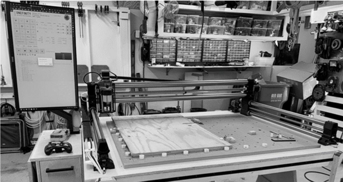
Figure 1.2: Three-axis CNC milling machine equipped with a Marposs MEMS vibration sensor.
