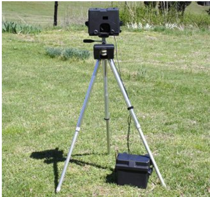
Figure 8. Digital camera setup from top to bottom: Canon 10D and housing, passive infrared receiver, and camera control unit (inside battery box).
