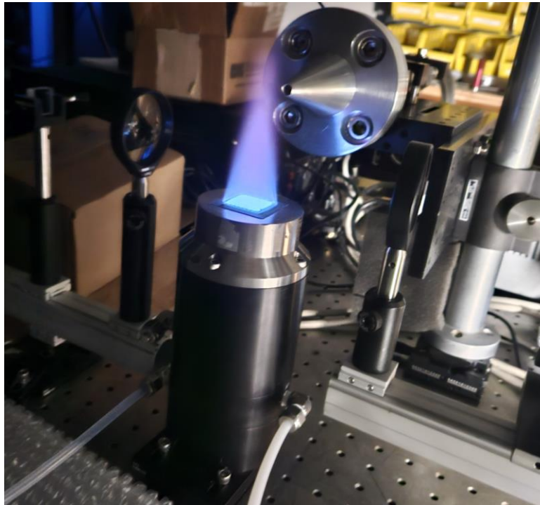
Figure 6.45. Mach 1.5, conical nozzle assembly and Hencken burner with flame in measurement region.
