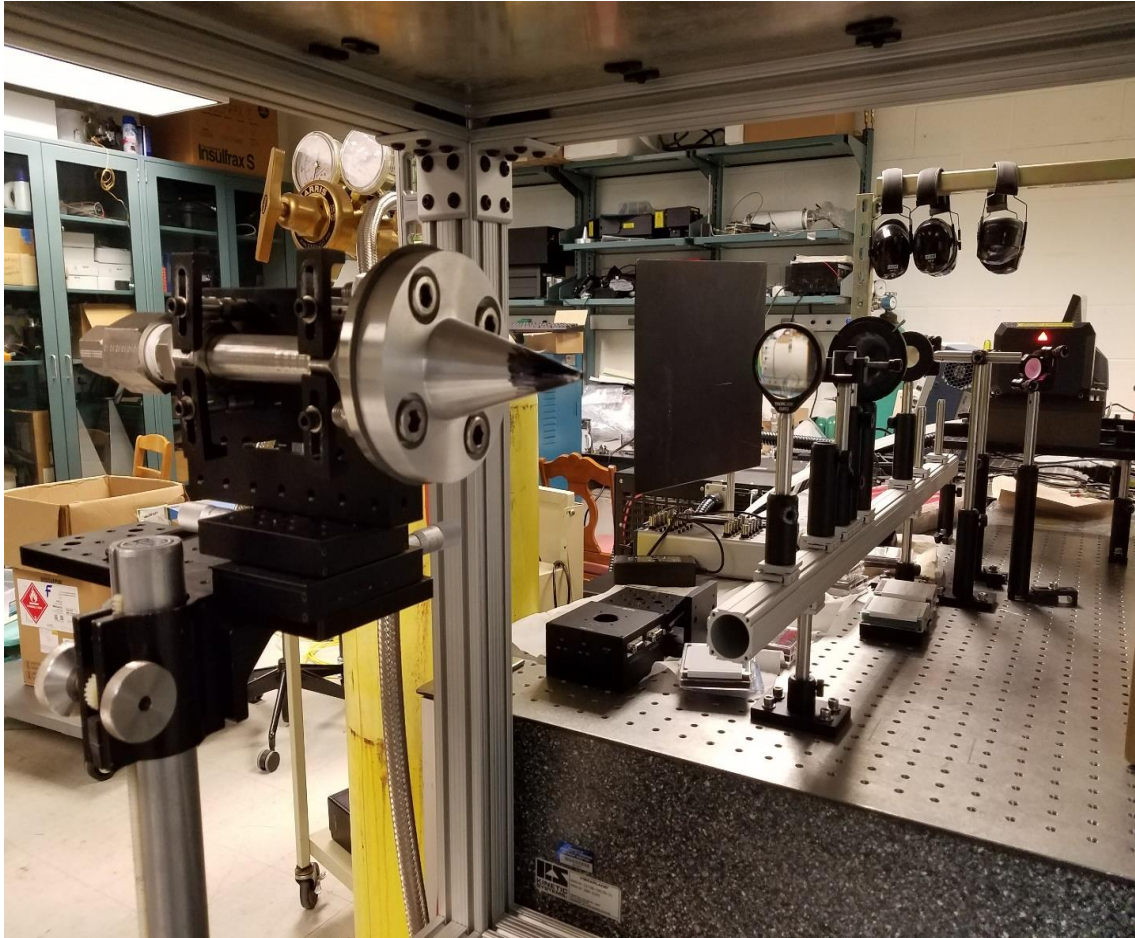
Figure A-2. Mach 1 jet nozzle assembly within test section in horizontal orientation.
