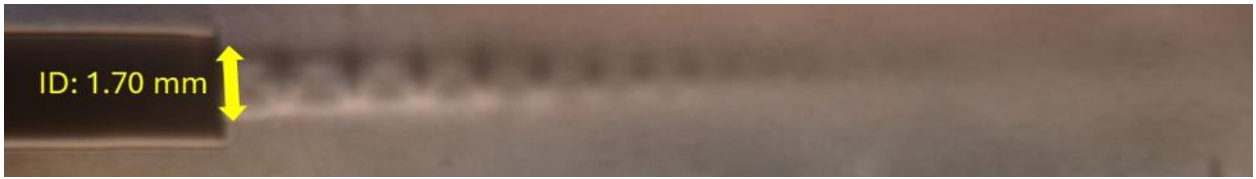
Figure 6.3. Schlieren image of underexpanded, free air jet with shock diamond structures.
