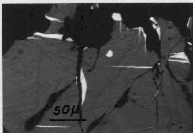
Figure 2.11. Mutual boundary and lamellar texture; Chino, New Mex. (gray: bn; white: cpy).
