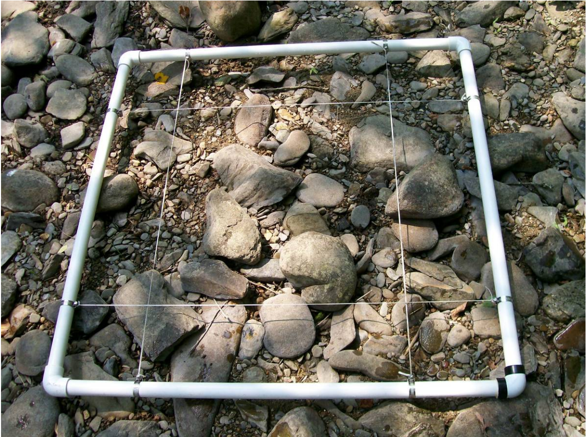
Figure 8. Design of PVC sampling frame. The frame was placed on the stream bank to provide a clearer picture of the design. Measurements were taken in stream.
