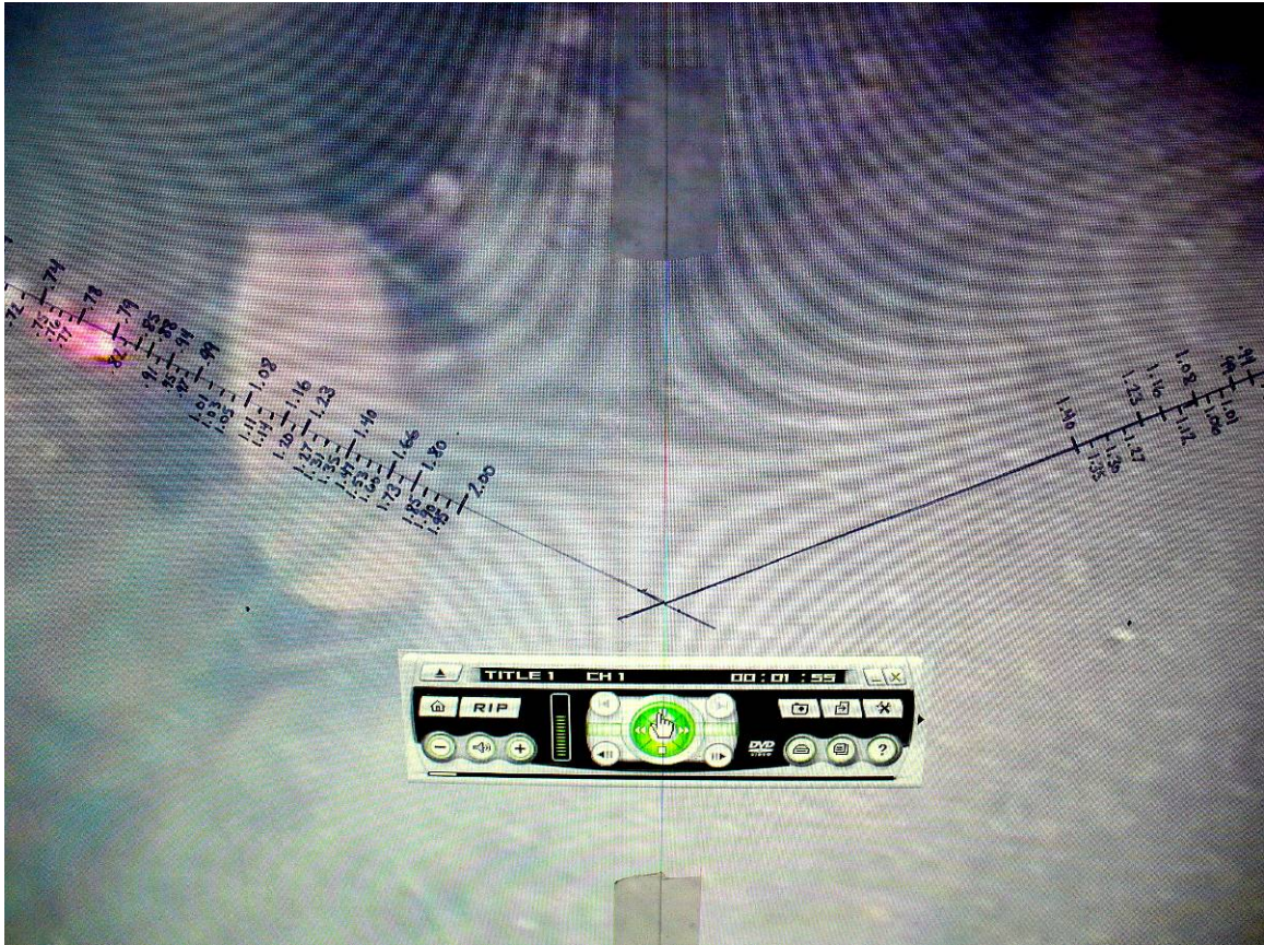
Figure 5. Acetate template sheet with conversion factors. Sheet is overlaid on a monitor showing video of substrate. A laser point can be seen on the left of the screen at about the 0.79 conversion factor. The AVS DVD player control panel can be seen at the center of the screen below the sample point.
