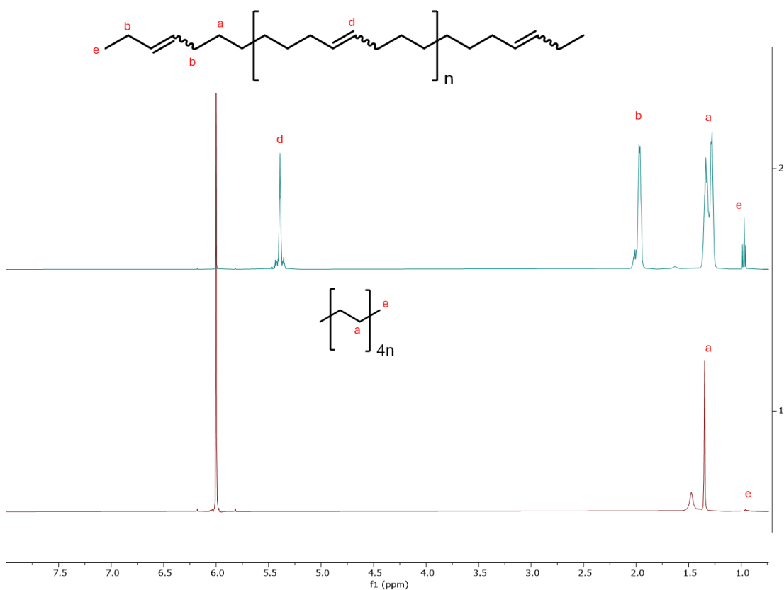
Figure 2.7 Stacked ^1\text{H} NMR spectra of polyethylene arranged such that the top is before hydrogenation and the bottom is after hydrogenation taken in 1,1,2,2-tetrachloroethane.
