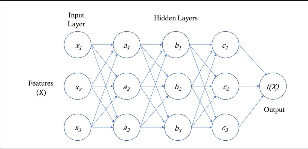
Figure 6. A fully connected neural network with three inputs and three hidden layers. The input layer consists of a set of neurons  $\{x_1, x_2, x_3\}$  representing the input features. Each neuron in the hidden layers applies a weighted linear transform, followed by a nonlinear activation function to the values it receives and feeds the result forward through the network. From the results of the final hidden layer, the output layer calculates a result classifying the original input.
