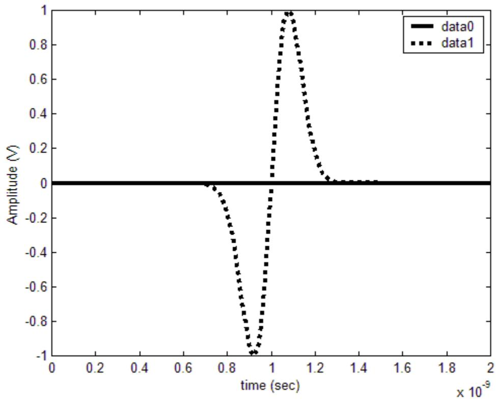
Figure 4.4: Gaussian first derivative pulse with OOK data.
