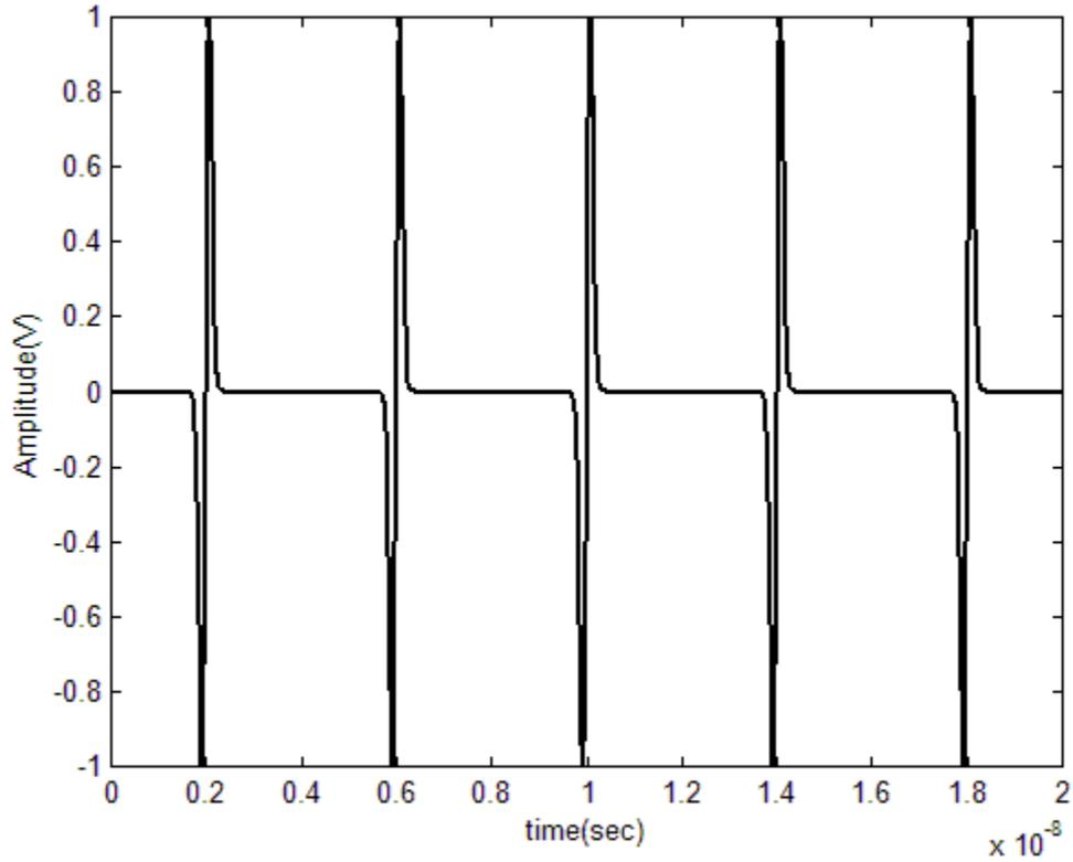
Figure 3.3: Gaussian first derivative pulse train of 5 monopulses.
