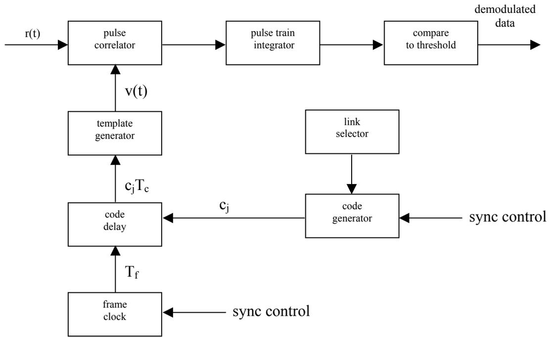
Figure 3.8: Block diagram of the UWB-IR receiver.
