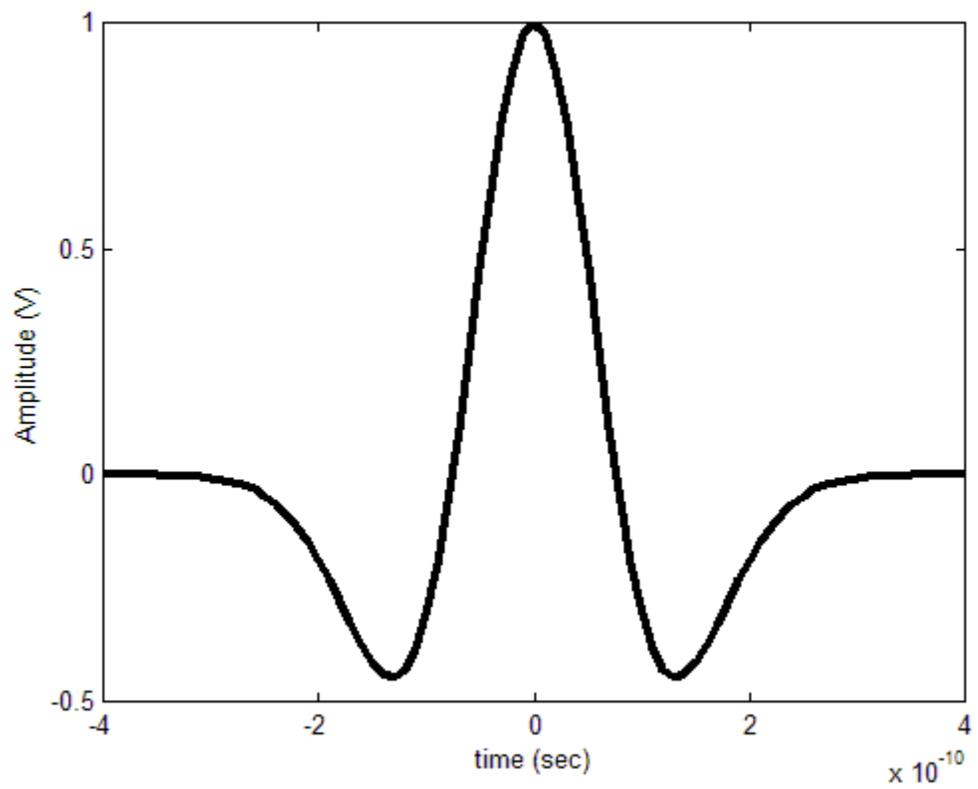
Figure 4.1: Gaussian second derivative pulse in time domain.
