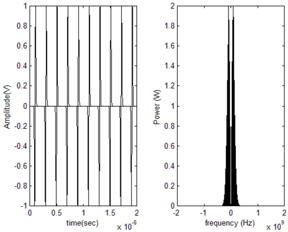
Figure 4.10: PSD of pulse train ( $N_s=10$ ).
