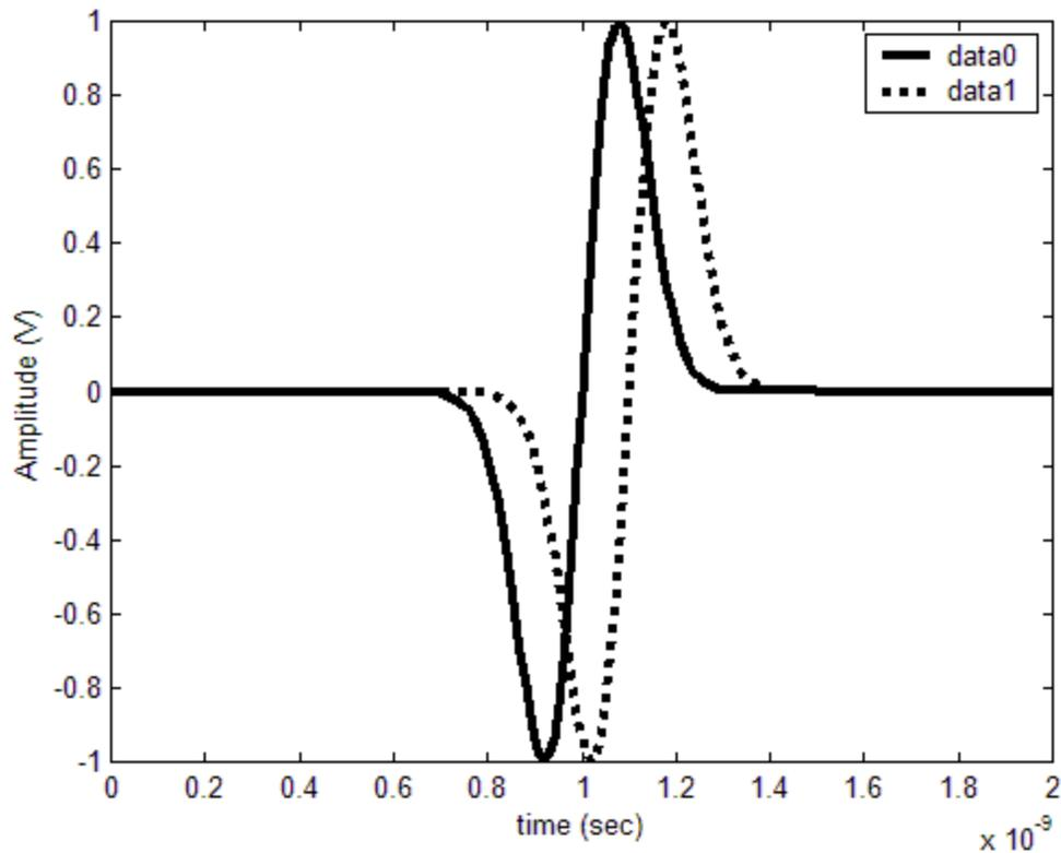
Figure 4.3: PPM data using Gaussian first derivative pulse.
