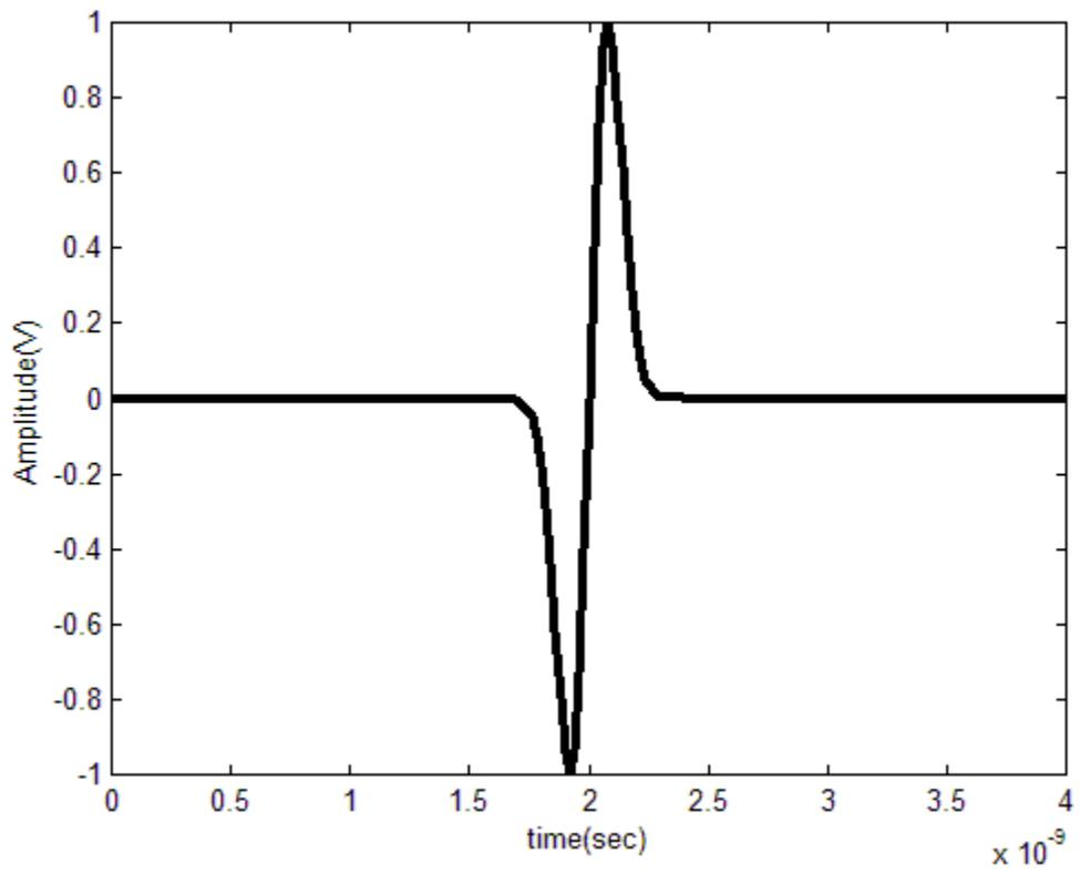
Figure 3.2: Gaussian first derivative pulse within a frame of  $T_f = 4\text{ns}$ .
