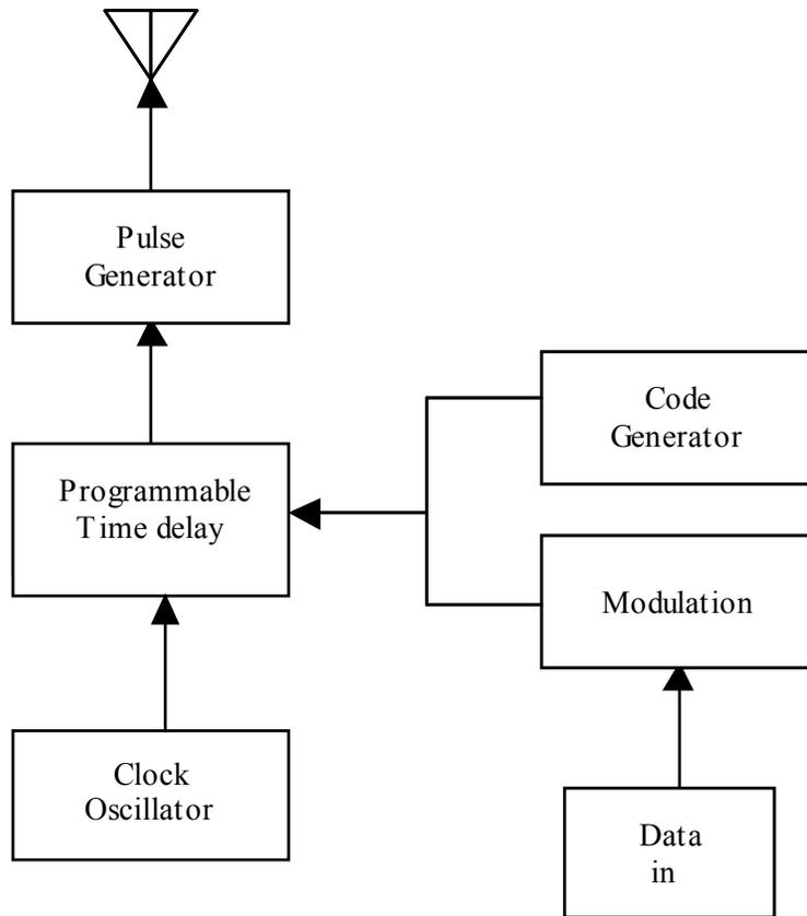
Figure 3.5: Block diagram of the UWB-IR transmitter.
