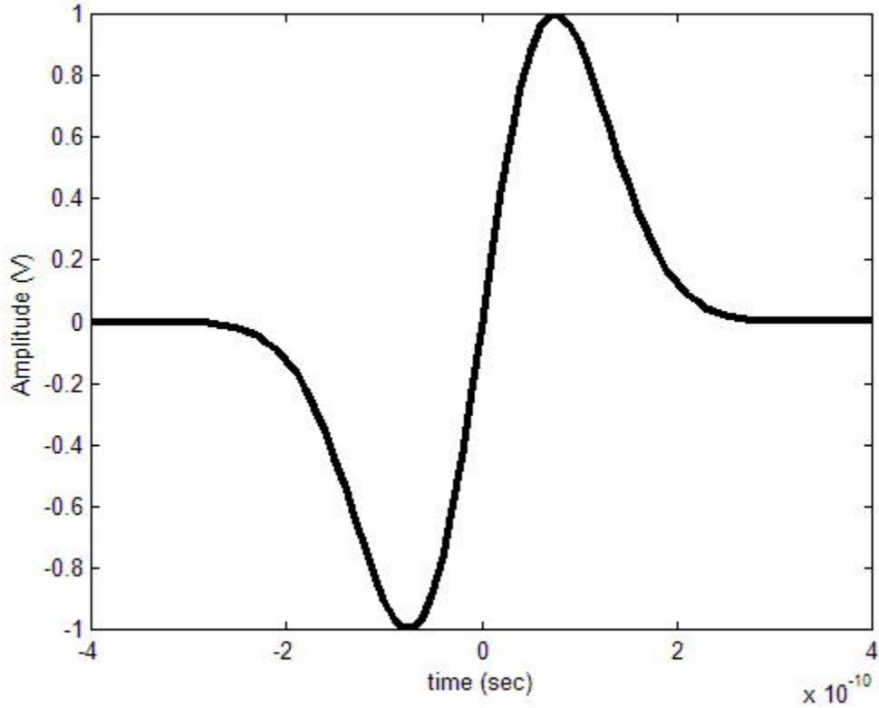
Figure 3.1: Gaussian first derivative pulse in time domain.
