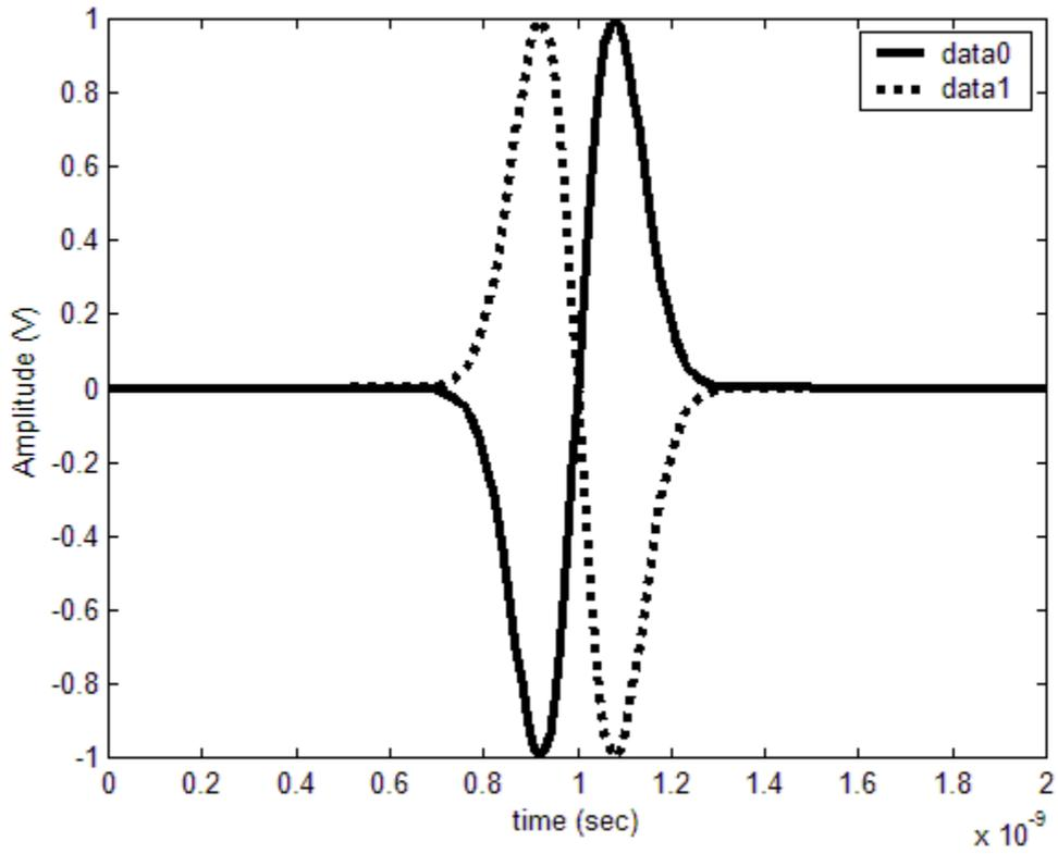
Figure 4.5: BPSK data with Gaussian first derivative pulse.
