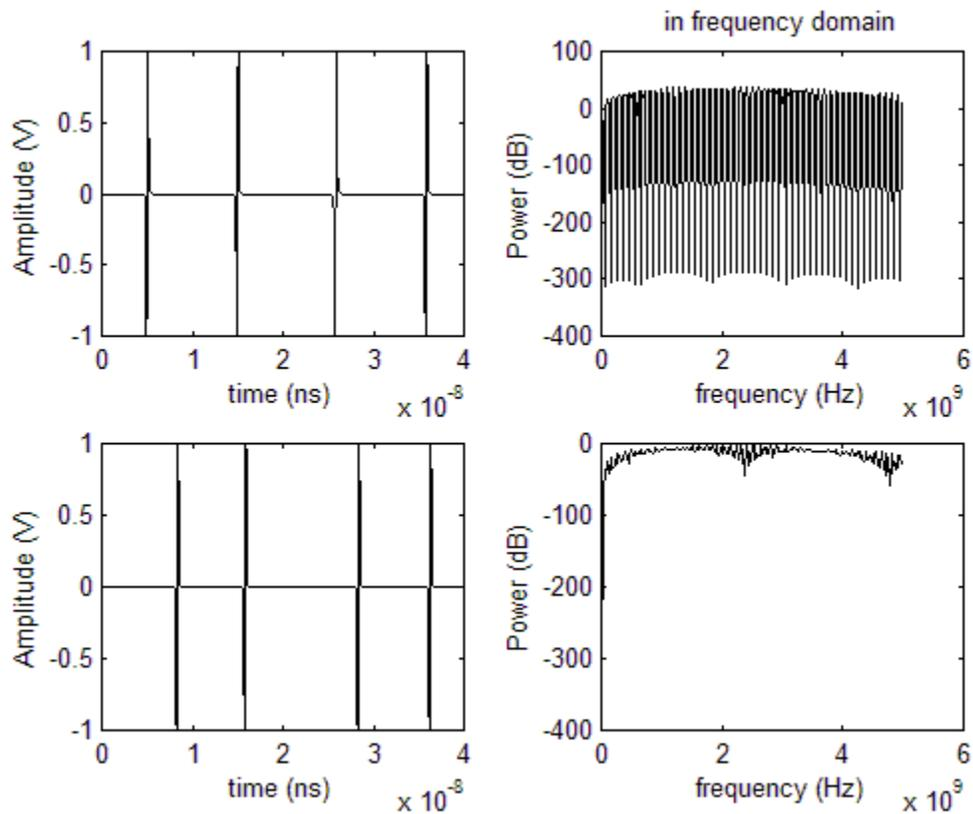
Figure 4.17: PSD of PPM with data [0 1] and code.
