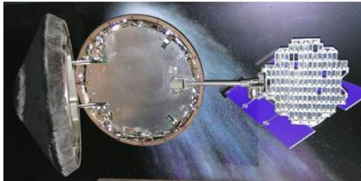
**Figure 2: Stardust Material Capture System**
