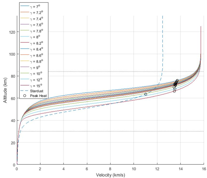
**Figure 8: Altitude Versus Velocity for Stardust Scaled to a 20 cm Diameter**
