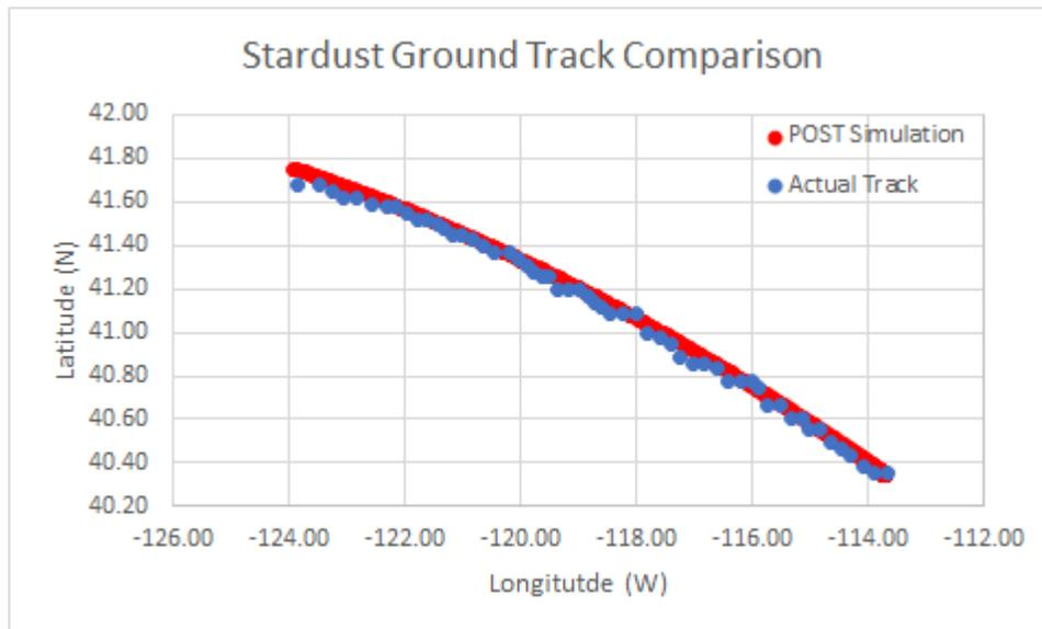
**Figure 4: Stardust Simulated Versus Actual Ground Track**
