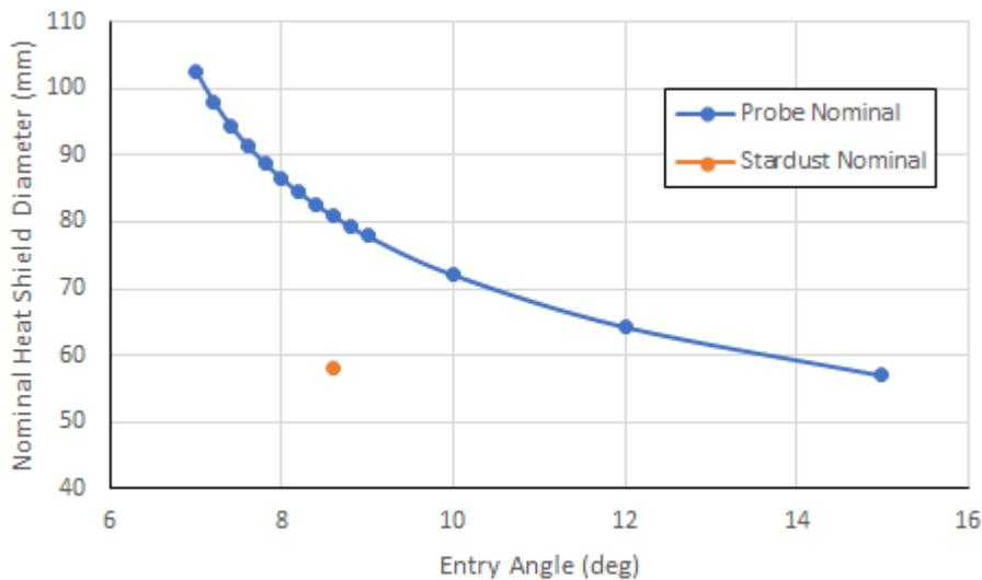
**Figure 14: 20 cm Probe Nominal Heat Shield Thickness Versus Entry Angle**
