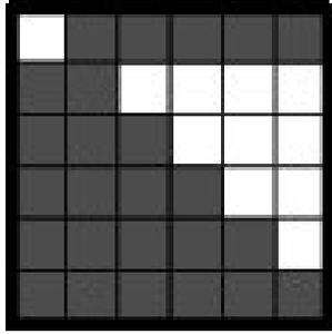
$$\begin{aligned} c_{0,0} &= d_{0,1} \oplus d_{0,2} \oplus d_{0,3} \oplus d_{0,4} \oplus d_{0,5} \\ c_{0,1} &= d_{0,0} \oplus d_{0,1} \\ c_{0,2} &= d_{0,0} \oplus d_{0,1} \oplus d_{0,2} \\ c_{0,3} &= d_{0,0} \oplus d_{0,1} \oplus d_{0,2} \oplus d_{0,3} \\ c_{0,4} &= d_{0,0} \oplus d_{0,1} \oplus d_{0,2} \oplus d_{0,3} \oplus d_{0,4} \\ c_{0,5} &= d_{0,0} \oplus d_{0,1} \oplus d_{0,2} \oplus d_{0,3} \oplus d_{0,4} \oplus d_{0,5} \end{aligned}$$
