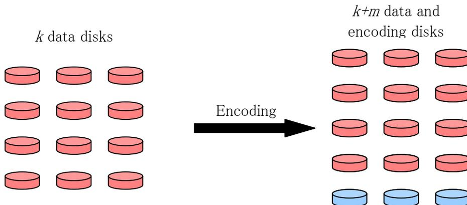
Figure 1: Encoding using an erasure code.
