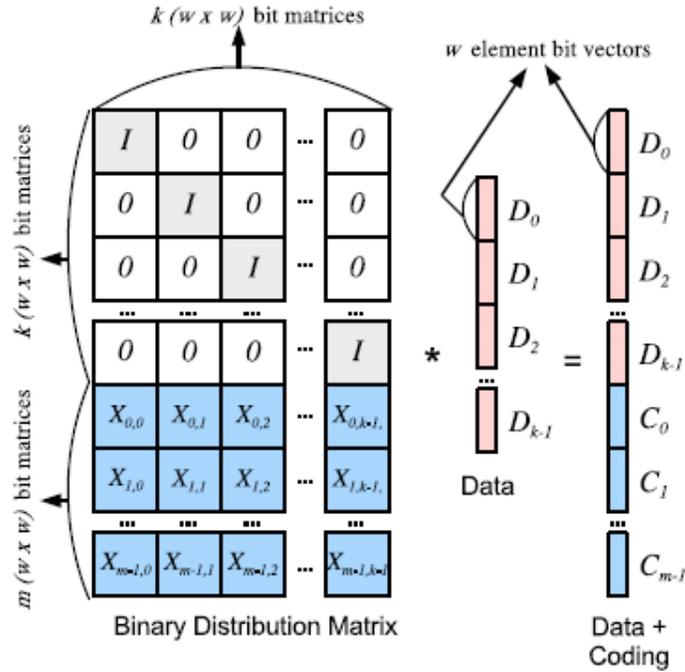
Figure 3: Bit-Matrix Encoding
