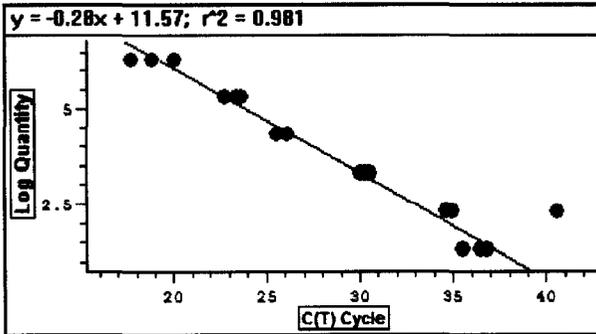
Figure 4. This graph shows the standard curve generated that allows for the calculation of the amount of DNA present in each sample.
