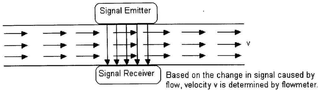
Figure 2. Perturbation of Known Electromagnetic or Ultrasonic Signal
