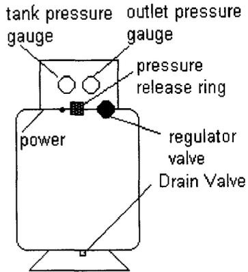
The Sears air compressor is capable of blowing large quantities of air at high flow rates, or gentle streams of air as desired. This air can be employed for a variety of purposes. The compressor can produce pressures as high as 130 psi, so caution is required in its operation. Below is a guide to the safe operation of the craftsman air compressor.
