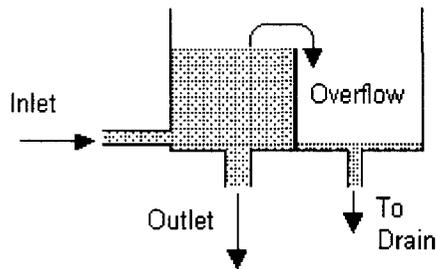
The inlet flow volume is purposefully made to be greater than the outlet flow volume, so there is a constant, predictable overflow into the overflow chamber. The amount of fluid in the primary chamber is therefore constant and at a constant height; therefore, the pressure at the outlet remains constant.
