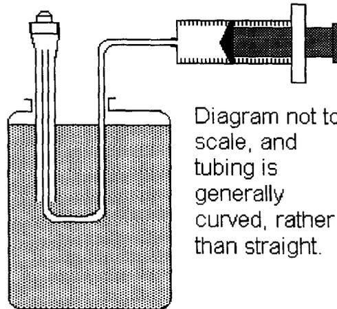
5. Draw out the trapped air with the syringe. If the syringe should fill with air, simply remove from the small diameter tubing while pinching the tubing shut and empty. Then reconnect and continue. It will probably be necessary to manipulate the thin tubing to be able to draw out all the trapped air. The use of a thin rod to hold the large diameter tubing probably will be helpful.
