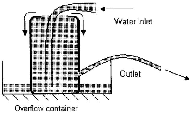
The overflow container was elevated to provide the pressure head through its height. The only drawback to this constant pressure tank was the overflow container not having a ready means of drainage.
