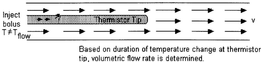
Figure 4. Injection of Fluid Bolus. Catheter (shaded) exaggerated for clarity.
