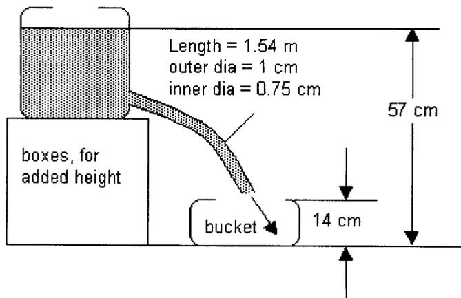
Allowing the water to run out of the tank for 1 min with an initial fluid height as shown, and measuring the amount of fluid flow caught in the bucket yielded the following data.
