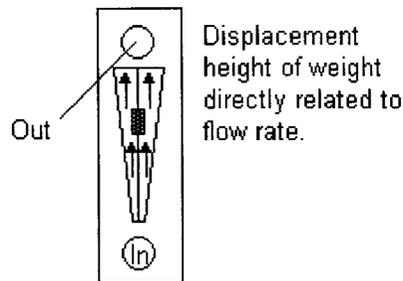
Figure 3. Flowmeter Based on Height Displacement of Known Weight in Special Tube
