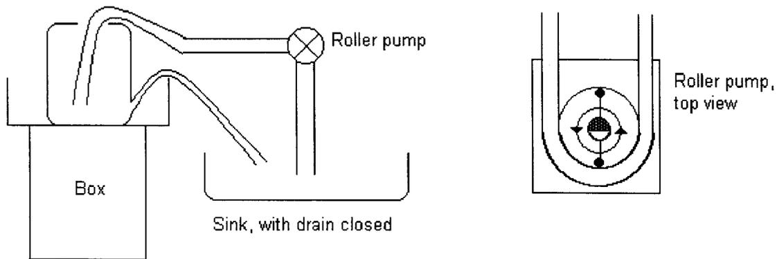
The overflow container was drained with one or more small diameter siphons back to the sink. It was found that the temperature of the water could be kept close to constant with periodic small additions of warm water. The roller pump was far less susceptible to air than the centrifugal pump, although its maximum output was less.
