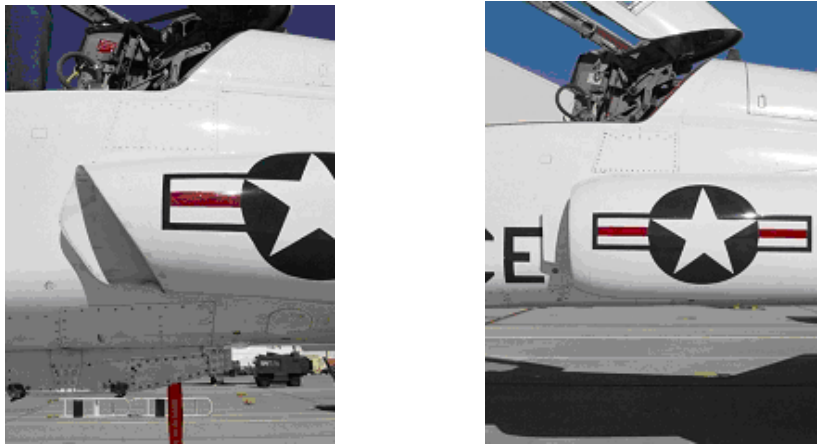
Figure 3. Comparison of non-modified (L) and modified (R) T-38 inlets.
