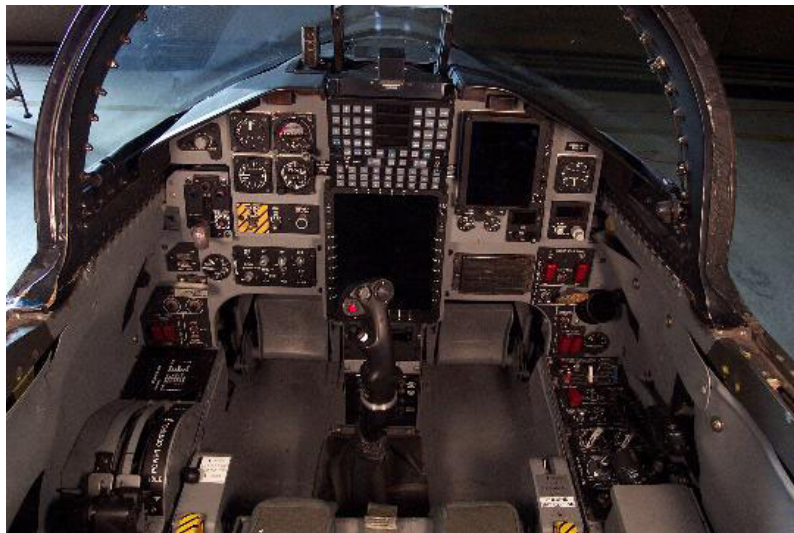
Figure 2. T-38C cockpit after the Avionics Upgrade Program.
