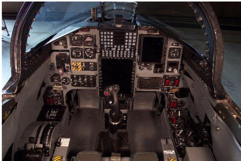
Figure 2. T-38C cockpit after the Avionics Upgrade Program.
