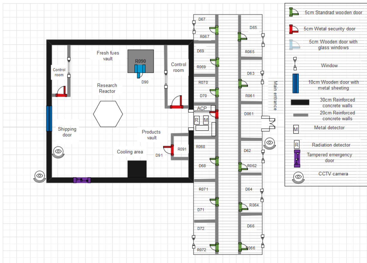
Figure 4: The New Research Reactor Building Floor Plan
