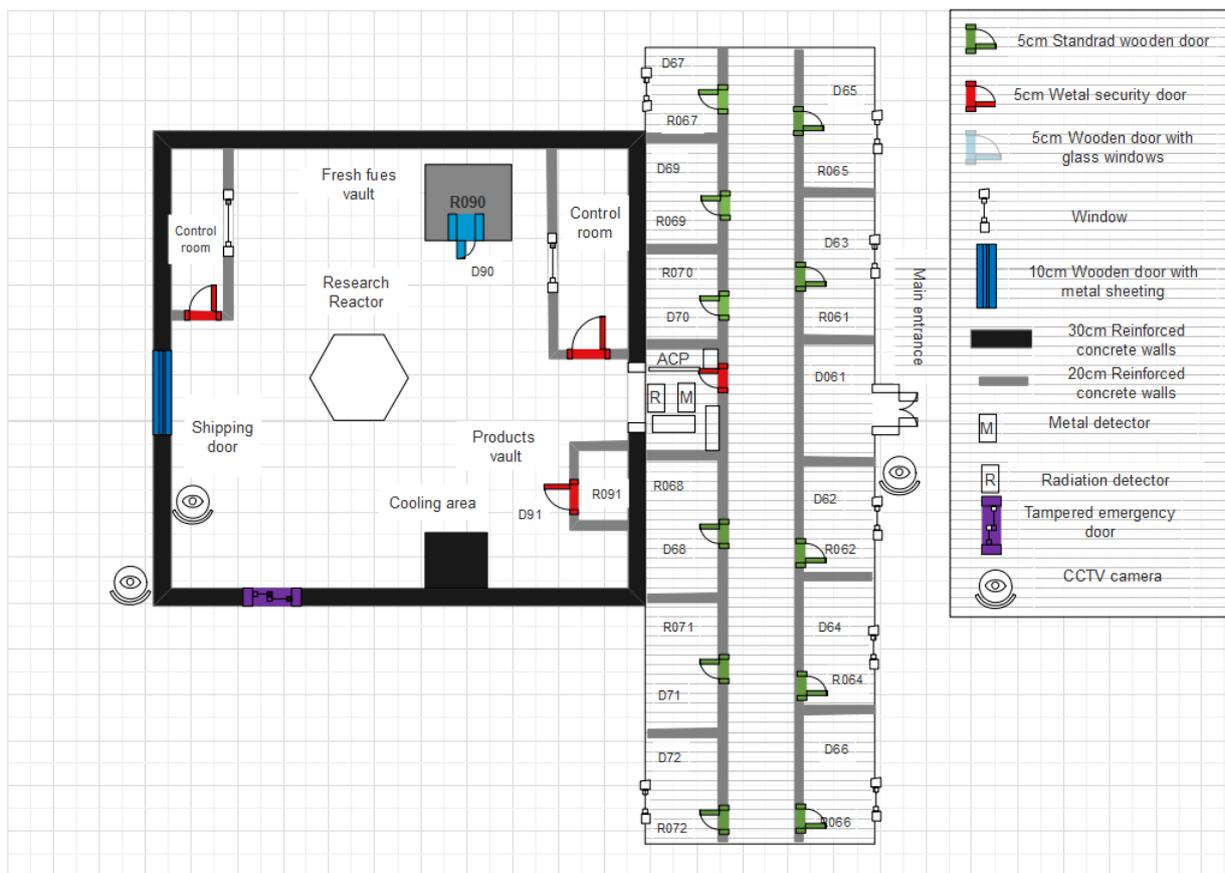
Figure 4: The New Research Reactor Building Floor Plan
