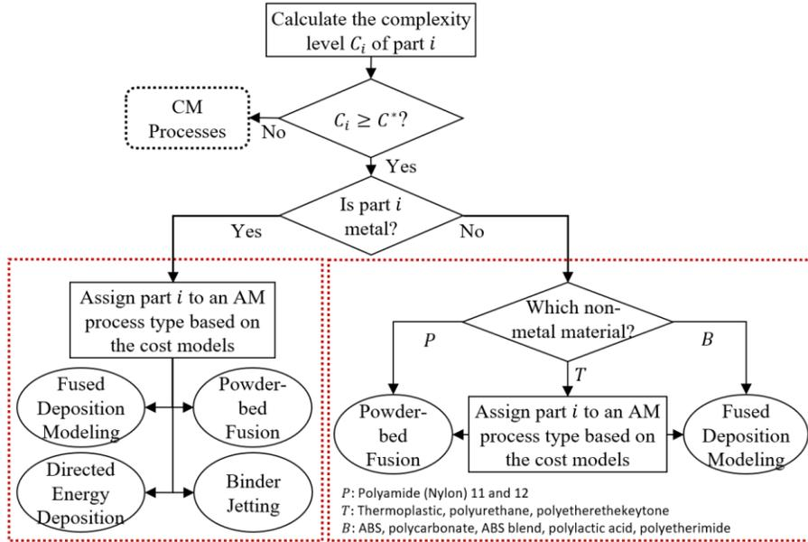
Figure 2.1 AM process selection framework.
