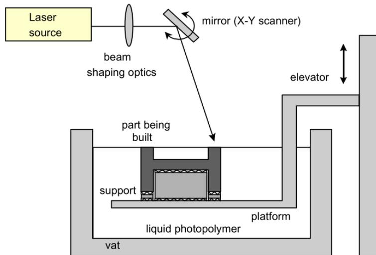
Figure 1.2 A schematic view of the stereolithography (Park et al., 1998)
