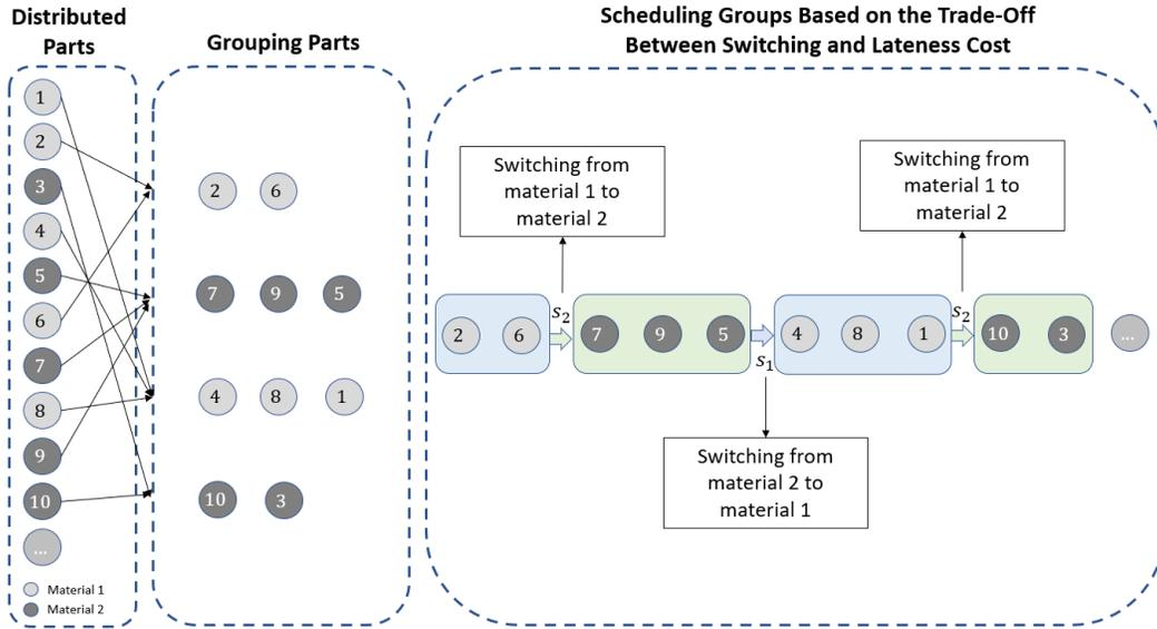
Figure 4.1 Demonstration of the proposed scheduling model
