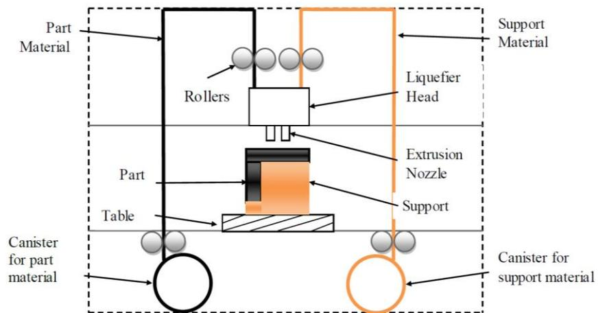
Figure 1.3 Schematic view of fused deposition modeling (Equbal et al., 2018)
