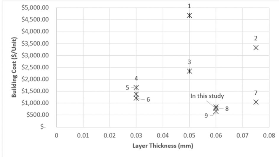
Figure 3.3 Changing in building cost depending on layer thickness settings.
