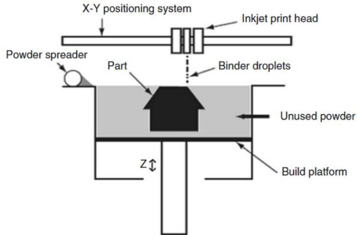
Figure 1.5 Schematic view of the binder jetting process (Kim et al., 2019)
