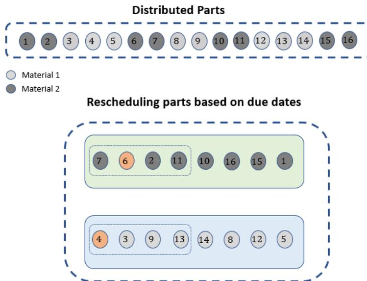
*Figure 4.4 Rescheduling parts based on the due dates until the late parts.*
