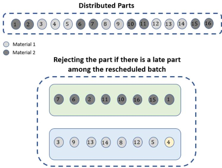
*Figure 4.5 Rejecting parts if there is a late part after re-sequencing parts based on the due dates.*
