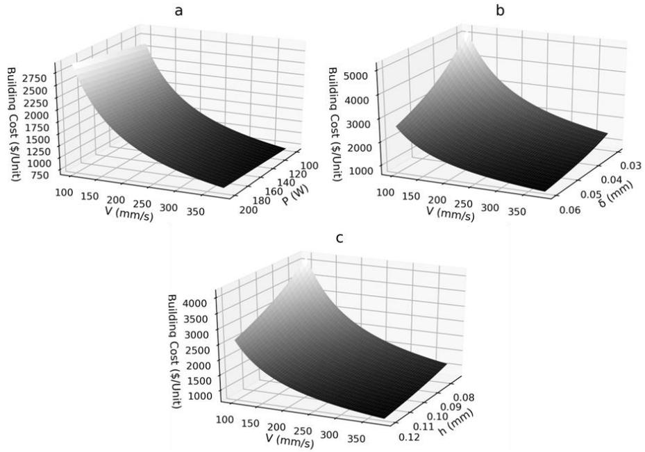
Figure 3.2 Changing in building cost depending on combination of scan speed and laser power (a), scan speed and layer thickness (b), scan speed and hatch distance (c)
