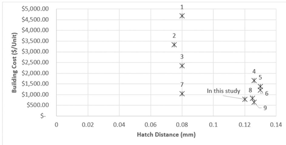
Figure 3.4 Changing in building cost depending on hatch distance settings.
