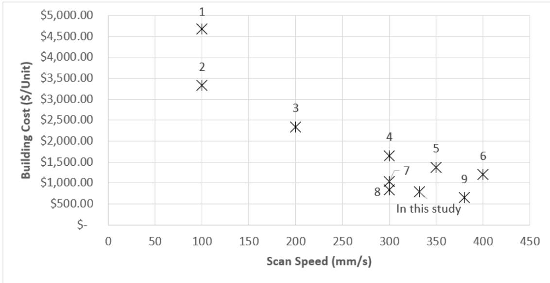
Figure 3.1 Changing in building cost depending on laser scan speed settings.
