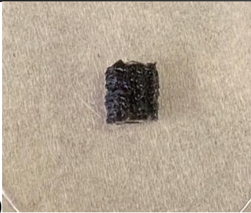
Figure 4.14 (a)Both constructs showed limited weight loss that could be explained by the crystal formation on the PLGA by the PBS. (b)PLGA+LOG at start. (c)at 8-week time point of degradation in dynamic bioreactor.
