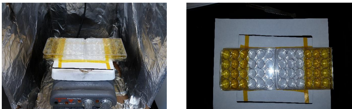
Figure 2.2 Air spray setup for graphene coatings on 24-well plates
