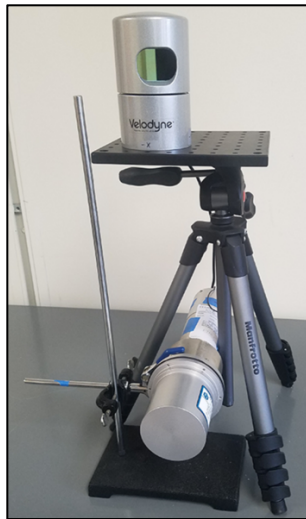
Figure 18: Velodyne LIDAR and radiation detector configuration at the University of Florida. [76]
