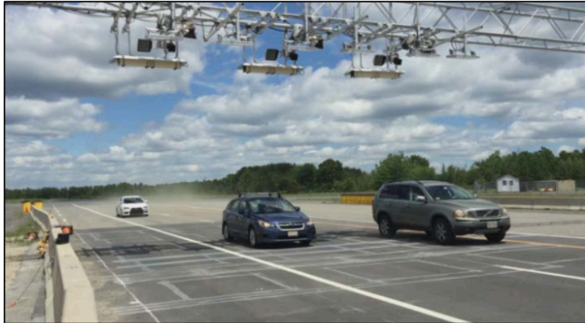
Figure 11: Testbed for DHS-RAIN showing license plate readers position above flowing traffic. [64]
