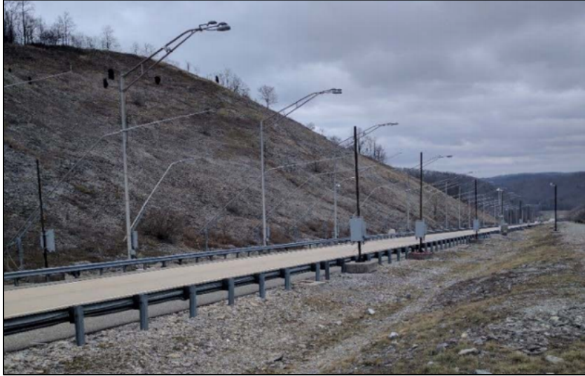
Figure 10: Testbed for DHS-RAIN with radiation detection sensors and video cameras along a roadway. [64]
