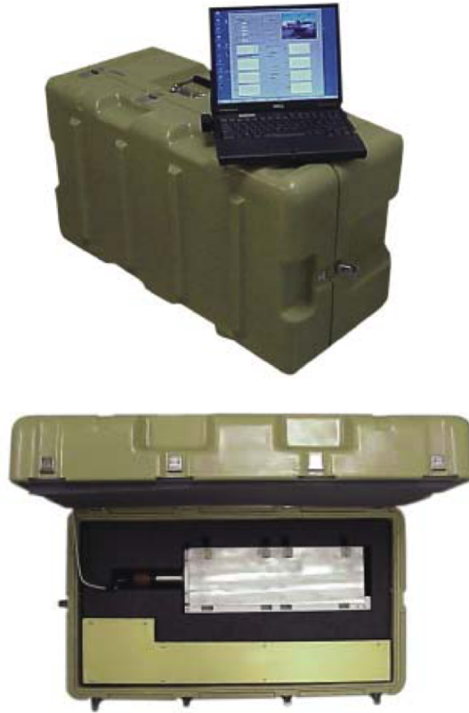
Figure 8: Image of the LLNL Adaptable Radiation Area Monitor system. [58]
